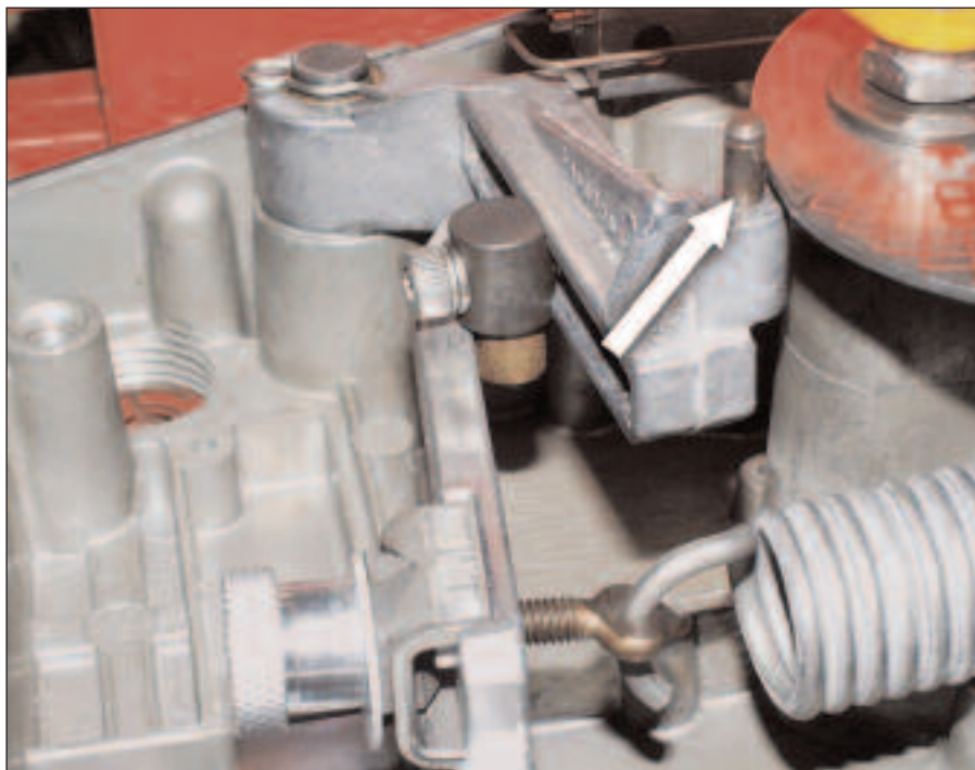
Figure 4. Closeup of feedback linkage inside positioner showing bearing roller failure
