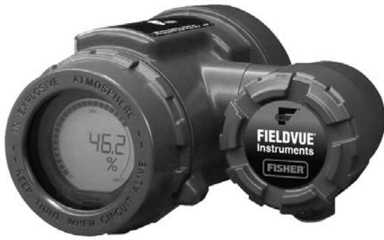
Figure 2-17. The FIELDVUE DLC3010 digital level controller is used with level sensors to measure liquid level, the level of the interface between two liquids, or liquid specific gravity (density). Changes in level or specific gravity exert a buoyant force on a displacer, which rotates a torque tube shaft. The digital level controller converts this rotational motion to an electronic signal that is used by a control valve to maintain the level or specific gravity set point.
