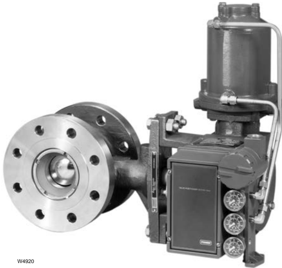
Figure 2-10. The 3620JP is an electro-pneumatic positioner that combines the functions of transducer and positioner into one unit. The combustion unit generally is more economical but may not be as flexible as separate units.
