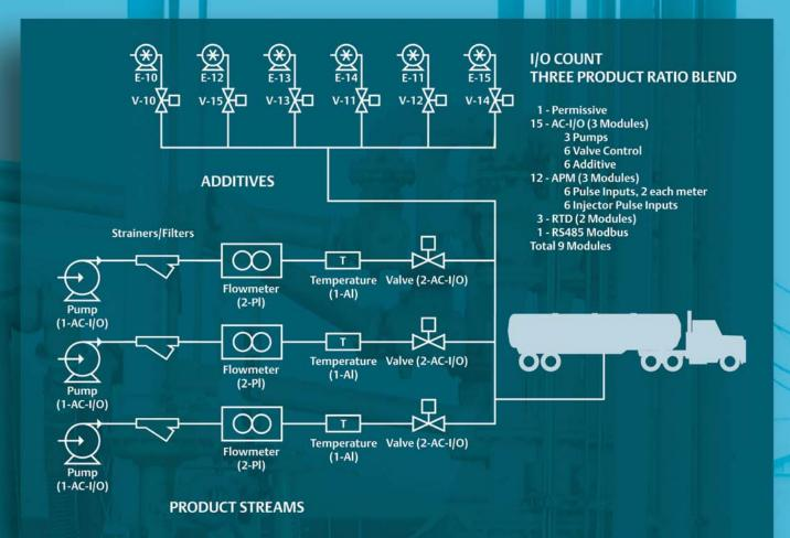
The DL8000 is capable of performing all blending, measurement, control, and monitoring needed to provide highly productive and rapid operations for most common loading configurations used in the industry.
