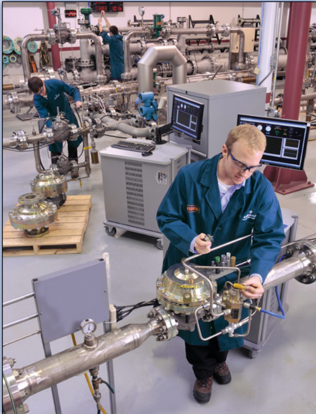
Testing the Type EZH with Whisper Trim ™ Noise Attenuation Technology in Emerson's flow laboratory in McKinney, Texas.
