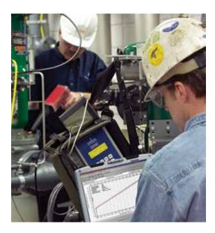
The portable FlowScanner 6000 is used to evaluate current operating conditions without having to disassemble or remove your control valves from the process. The FlowScanner system is flexible enough to run a variety of tests, including:
