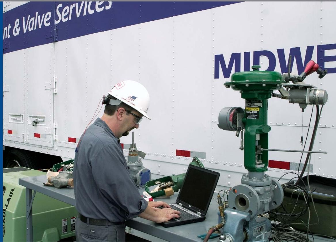
Emerson's **FlowScanner™ 6000** is a valve diagnostic system that conducts inline testing of valves, eliminating the need to remove and reinstall, to save you time and money. Valves are tested to manufacturing specifications, ensuring maximum performance and efficiency.
