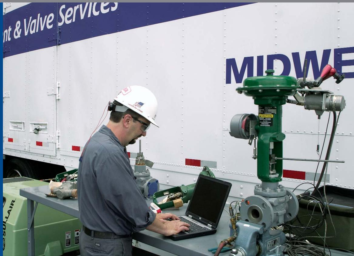
Emerson's **FlowScanner™ 6000** is a valve diagnostic system that conducts inline testing of valves, eliminating the need to remove and reinstall, to save you time and money. Valves are tested to manufacturing specifications, ensuring maximum performance and efficiency.
