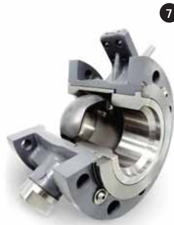
V150S erosion-resistant trim components protect the body from erosive wear and are retained without the use of press fits or threads for easy replacement.
