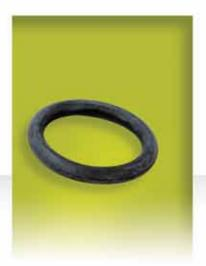
Specially formulated Fisher O-rings for spring-and-diaphragm and piston actuators have a solid lubricant dispersed throughout their cross section. As these O-rings wear, new lubricant is exposed, which maintains static and dynamic friction coefficients for consistent, smooth operation.
