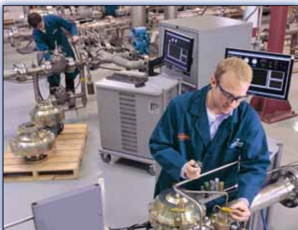
Testing the Type EZH with noise attenuation technology in Emerson's technical center in McKinney, Texas.
