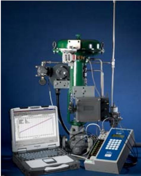
**Figure 2.** The FlowScanner 6000 set up to test and diagnose a sliding stem valve (left) and a rotary valve (below).
