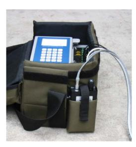
**Figure 1.** The FlowScanner 6000 housed in its convenient padded canvas operating bag, with the Interface module integrated into the accessory pocket (left). Shown with cables coiled and ready for transport (below).
