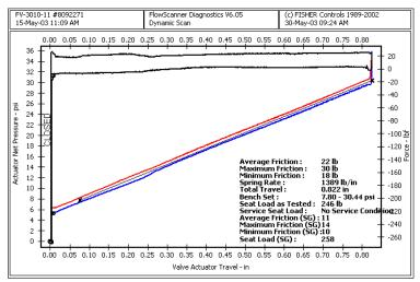
Figure 5. Strain gauge analysis overlaid on a net pressure plot. (Obtained using the SGIM-1 Strain Gauge Interface and the FlowScanner 6000 using a Teledyne QSS stem sensor.)
