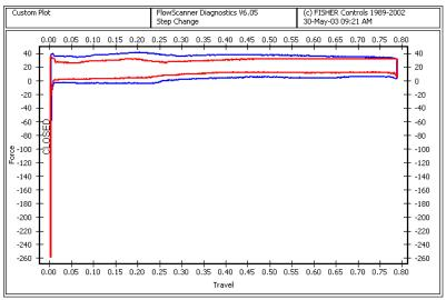
Figure 6. Overlay of a stepped open/close stroke compared to a controlled ramp stroke.
