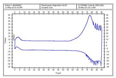
*Figure 7*. Plot of torque vs. travel for a rotary valve with QSS sensor.
