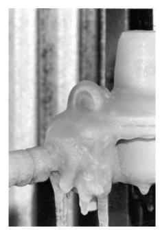
*Figure 4.* Vents on horizontally mounted regulators became quickly plugged during Fisher's tests.
