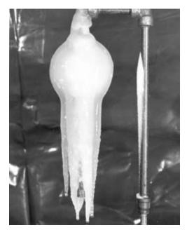
**Figure 2.** Ice completely covered the regulator Fisher Controls used in the freeze tests.
