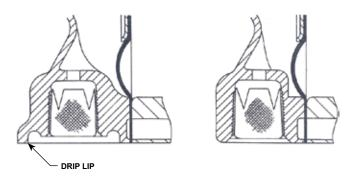
**Figure 1.** Drip lip vent construction has a recessed vent opening while the non-drip lip version on the right does not.
