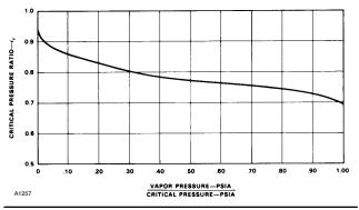
Use this curve for liquids other than water. Determine the vapor pressure/ critical pressure ratio by dividing the liquid vapor pressure at the valve inlet by the critical pressure of the liquid. Enter on the abscissa at the ratio just calculated and proceed vertically to intersect the curve. Move horizontally to the left and read the critical pressure ratio,  $r_c$ , on the ordinate.
