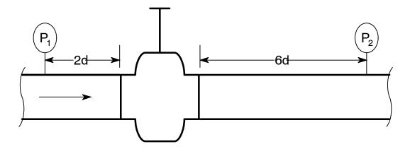
The control volume as defined by ISA 75.01.01 includes two diameters of piping upstream of the valve and six diameters downstream. This allows the fluid to fully develop prior to entry into the valve and enough time to recover downstream of the valve when  $C_V/d^2 \le 30$ . For these cases where  $C_V/d^2 > 30$ , alternative methods need to be considered.
