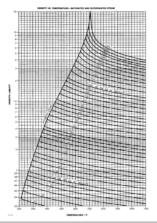
The degree of superheat is the difference between the actual temperature and the saturation steam temperature.
