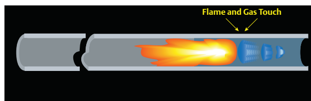
Figure 14. Concept of deflagration-to-detonation transformation in a pipe.
