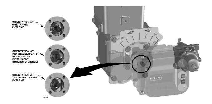
Figure 1. Magnet Assembly Orientation
