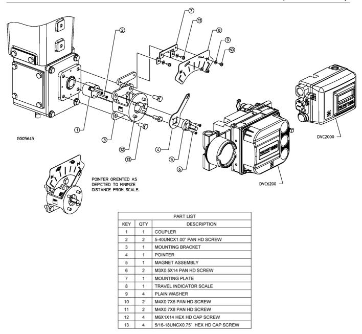
Figure 2. Mounting Parts Identification
