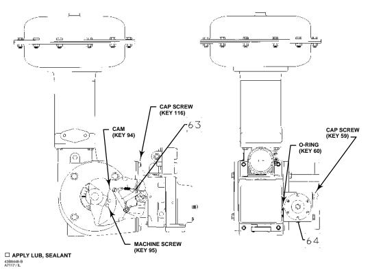
Figure 2. Type DVC5020 or DVC6020 Digital Valve Controller with Integrally Mounted Filter Regulator Mounted on Type 1051 Size 40 Actuator
