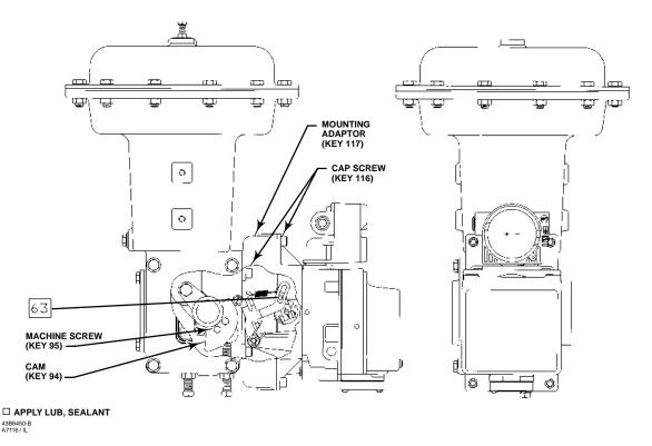
Figure 1. Type DVC5020 or DVC6020 Digital Valve Controller Mounted on Type 1052 Size 33 Actuator
