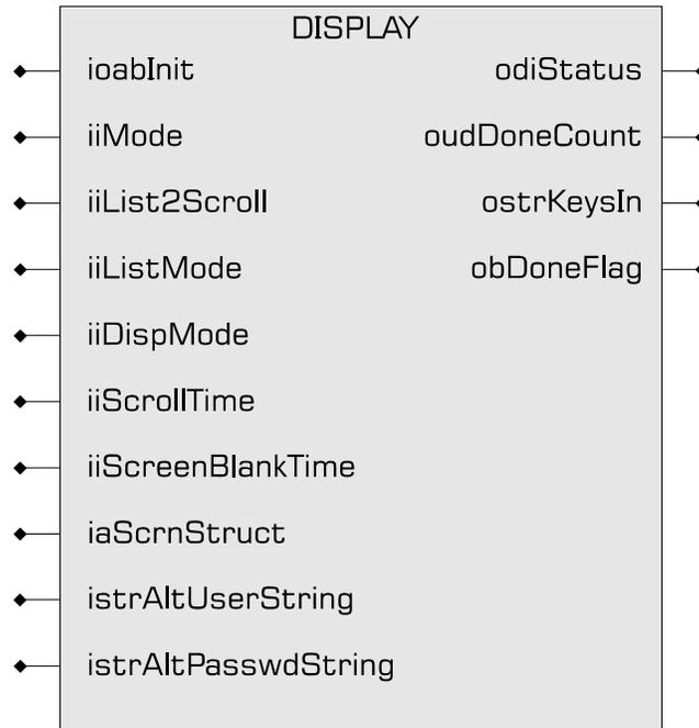
**Figure 2 - ACCOL3 DISPLAY Function Block Parameters**
