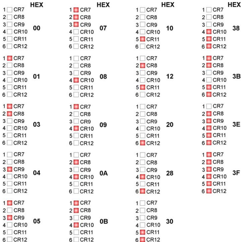
**Figure 6 – CW\_30 CPU Status LED Hexi-decimal Codes**
