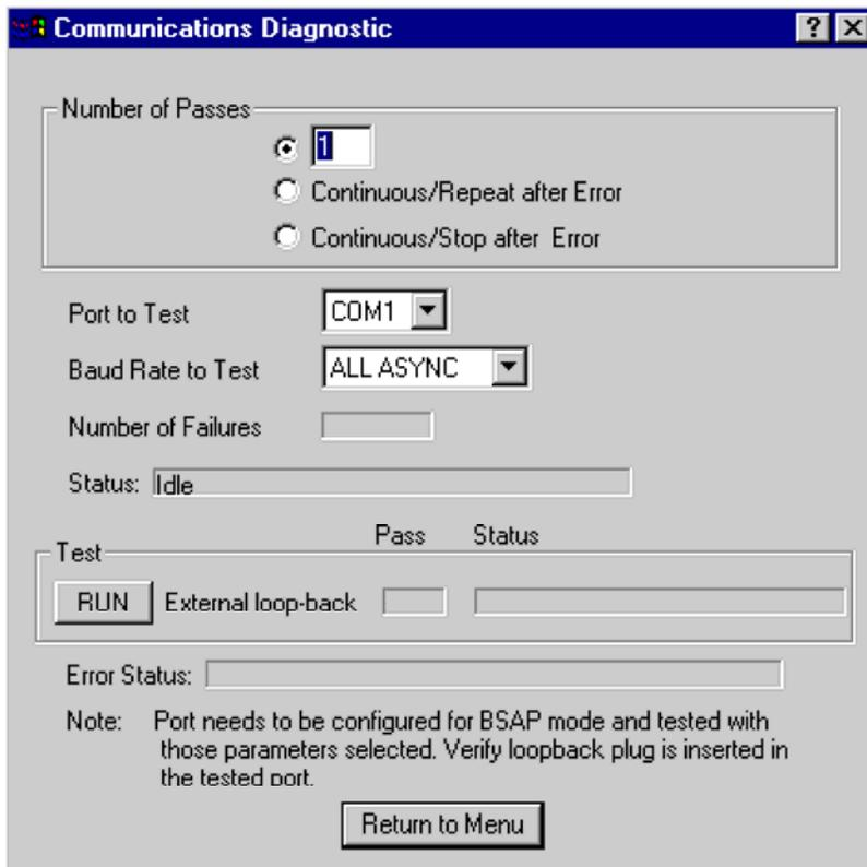
**Figure 24 - WINDIAG’s Communications Diagnostic Menu**
