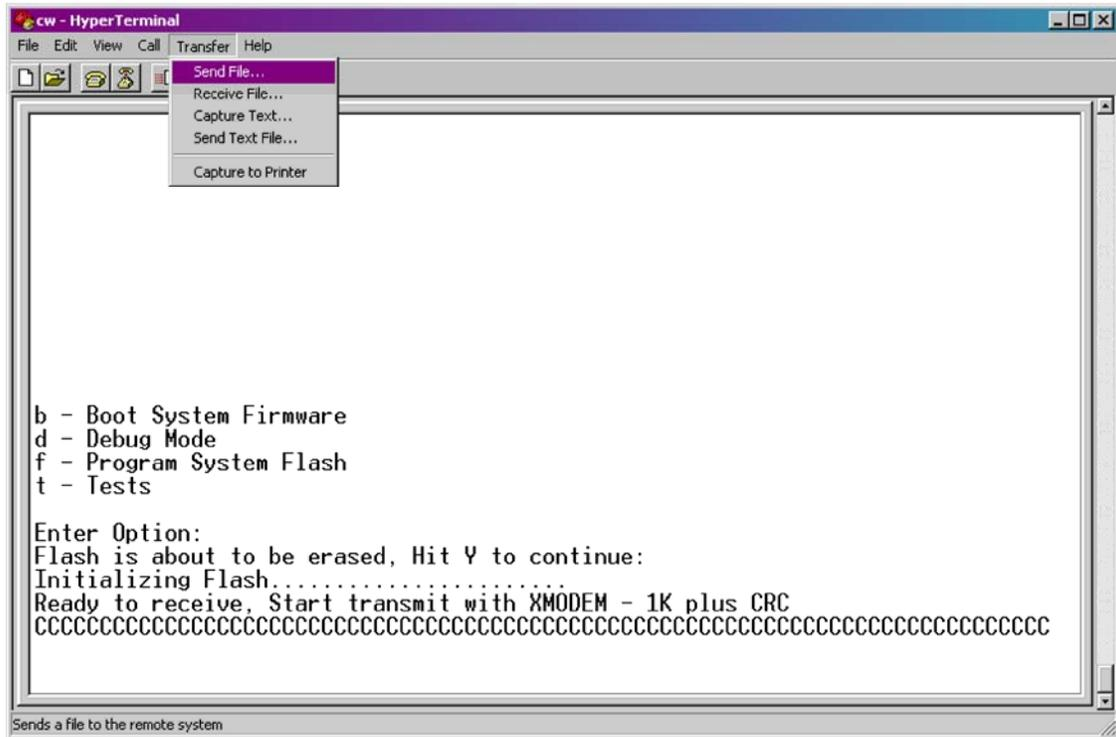
**Figure 17 - HyperTerminal FLASH Download Menu (Ready to Download) - (Transfer/Send File Selected)**
