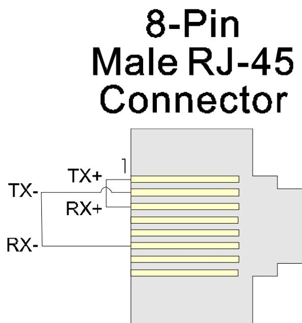
**Figure 26 - RJ-45 Ethernet Loop-back Plug**
