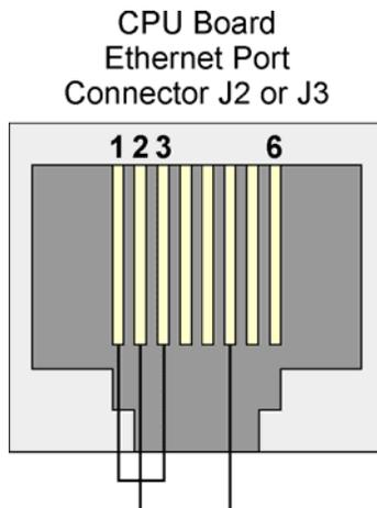
**Figure 5 - 10/100Base-T Connector (P2) with Cable Configured for Loopback**
