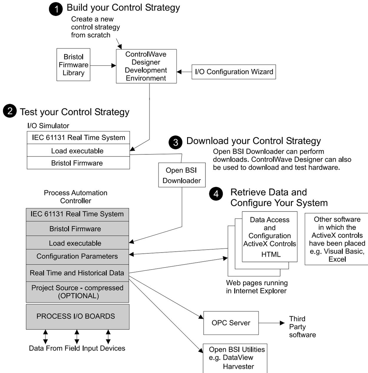
Figure 1 - ControlWave - Control Strategy Software Diagram
