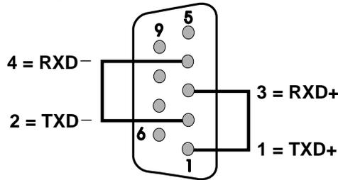
**Figure 23 - RS-485 Loop-back Wires**
