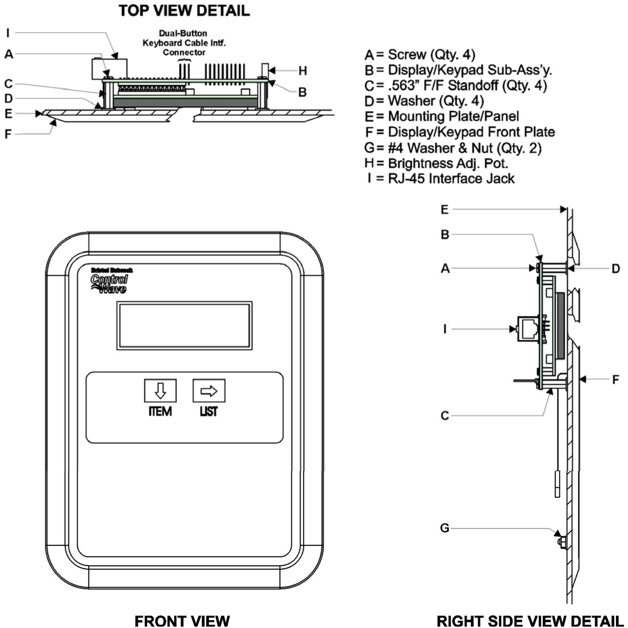
**Figure 27 - Dual-button Display/Keypad Assembly Installation Drawing**
