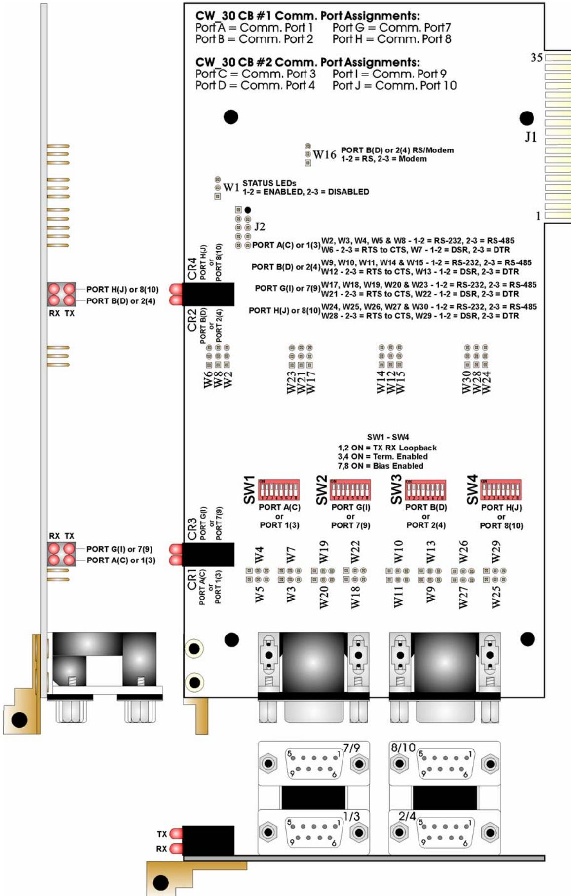
Figure 9 - CW\_30 - 4-Port CB Board Component Identification Diagram
