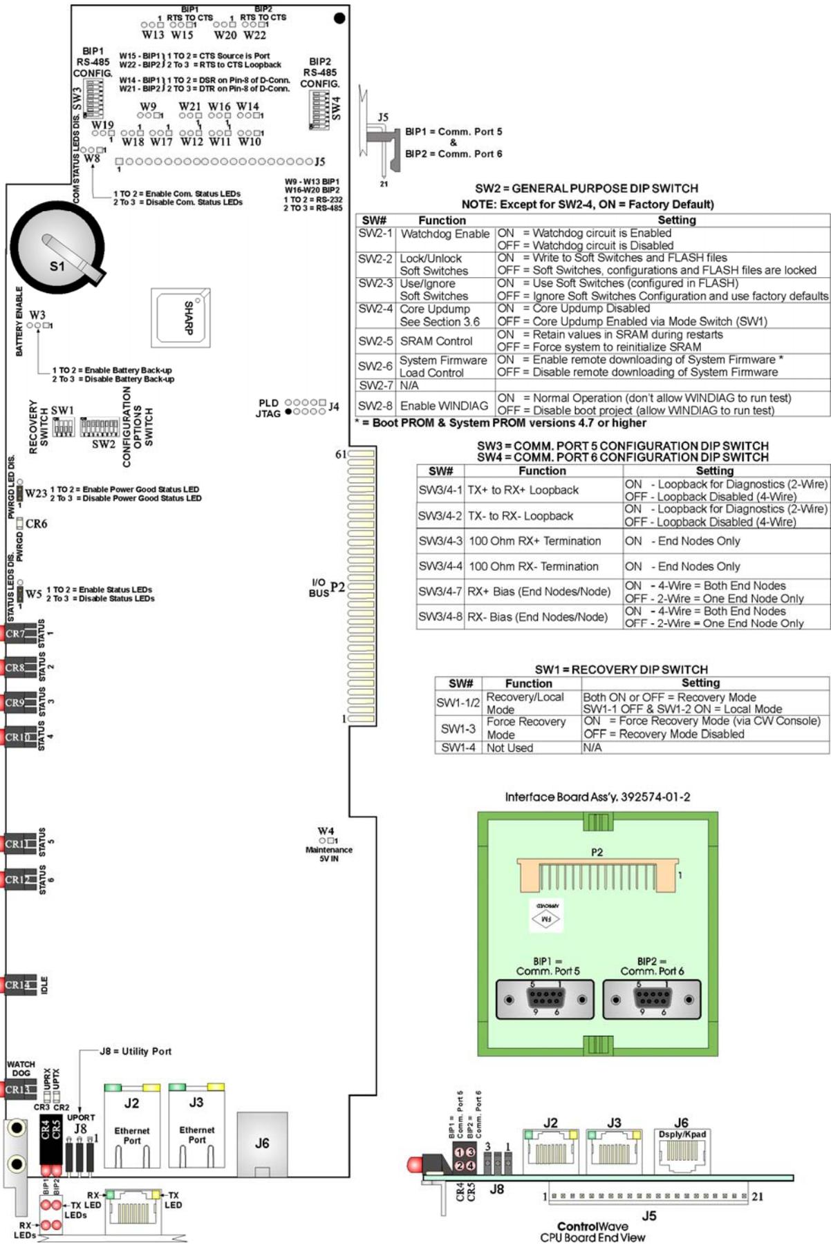
Figure 2 – CW\_30 CPU Board Component Identification Diagram
