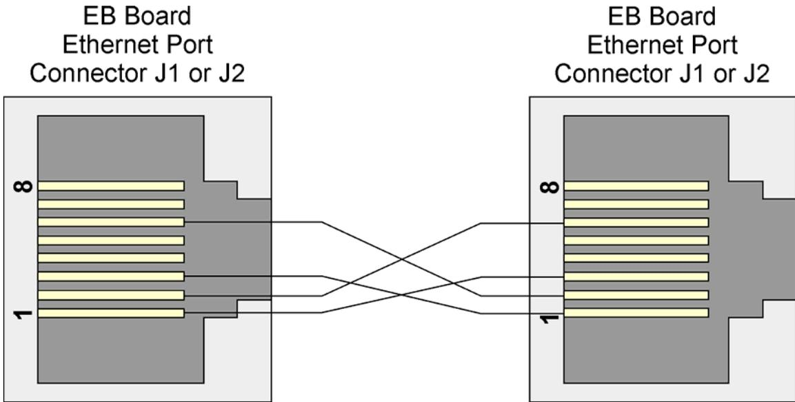
**Figure 3 - Point-to-Point 10/100Base-T Ethernet Cable**
