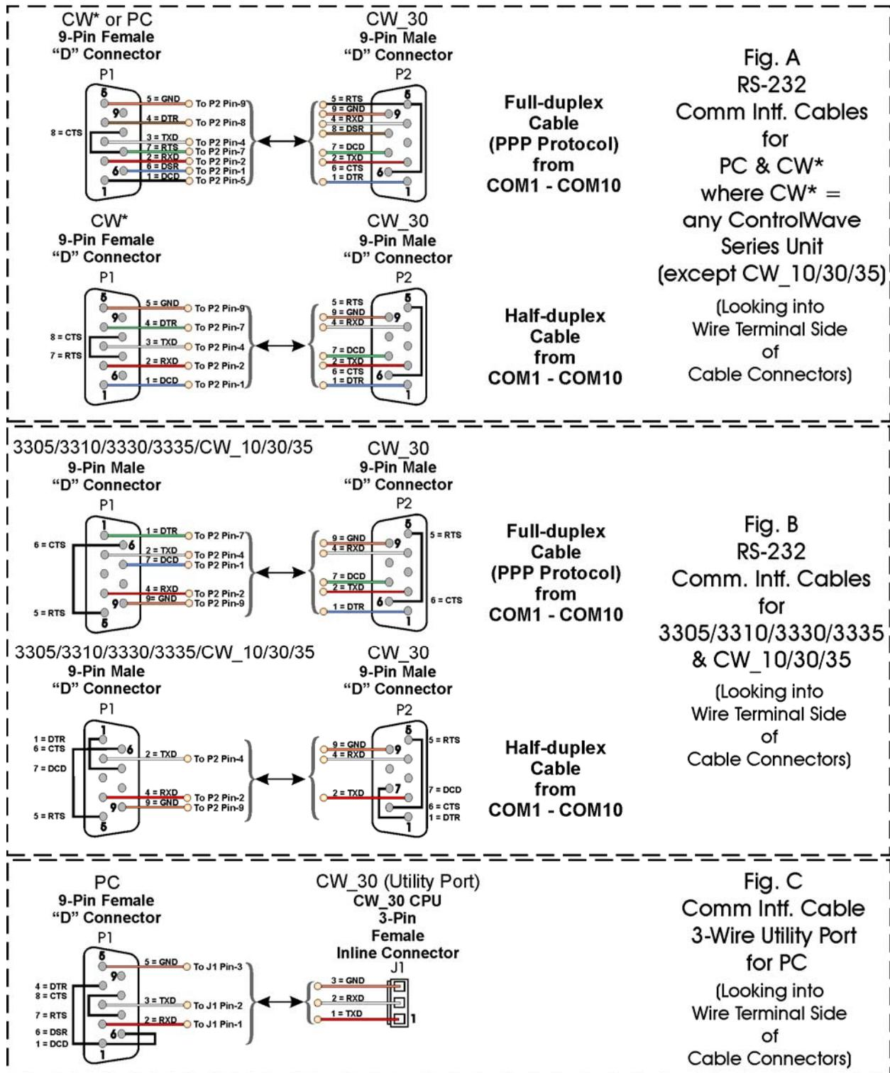
Figure 10 - Communication Port RS-232 Cable Wiring Diagram
