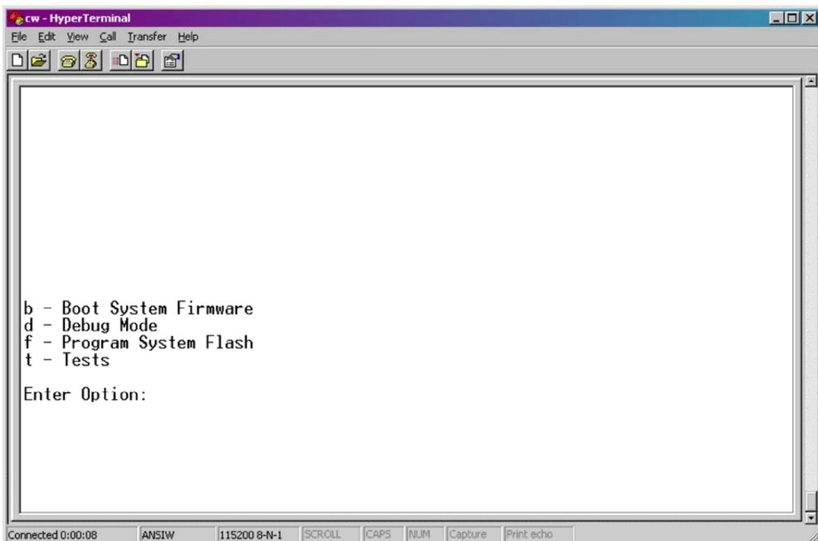
**Figure 16 - HyperTerminal Recovery Mode Menu**
