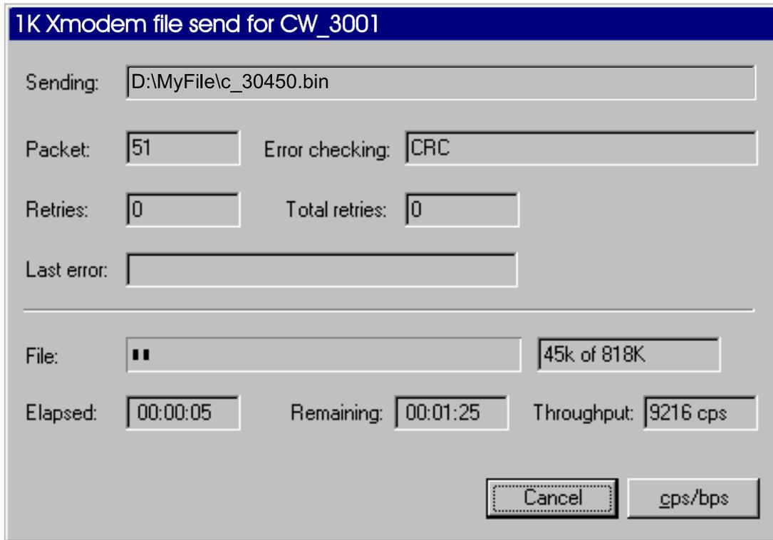
**Figure 19 - HyperTerminal FLASH Download (Download in Process)**
