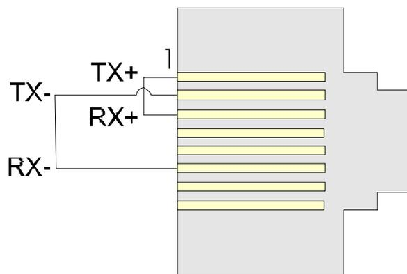
**Figure 28 - RJ-45 Ethernet Loop-back Plug**
