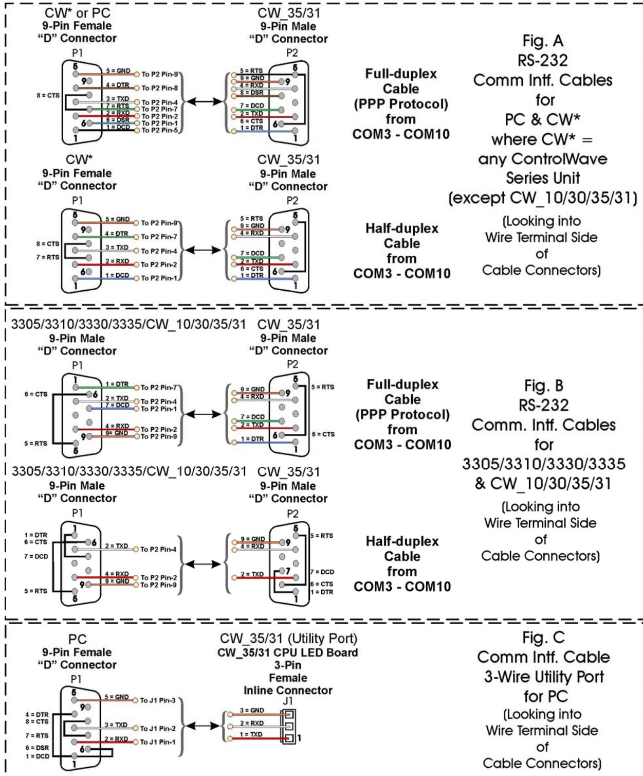
Figure 12 - Communication Port RS-232 Cable Wiring Diagram
