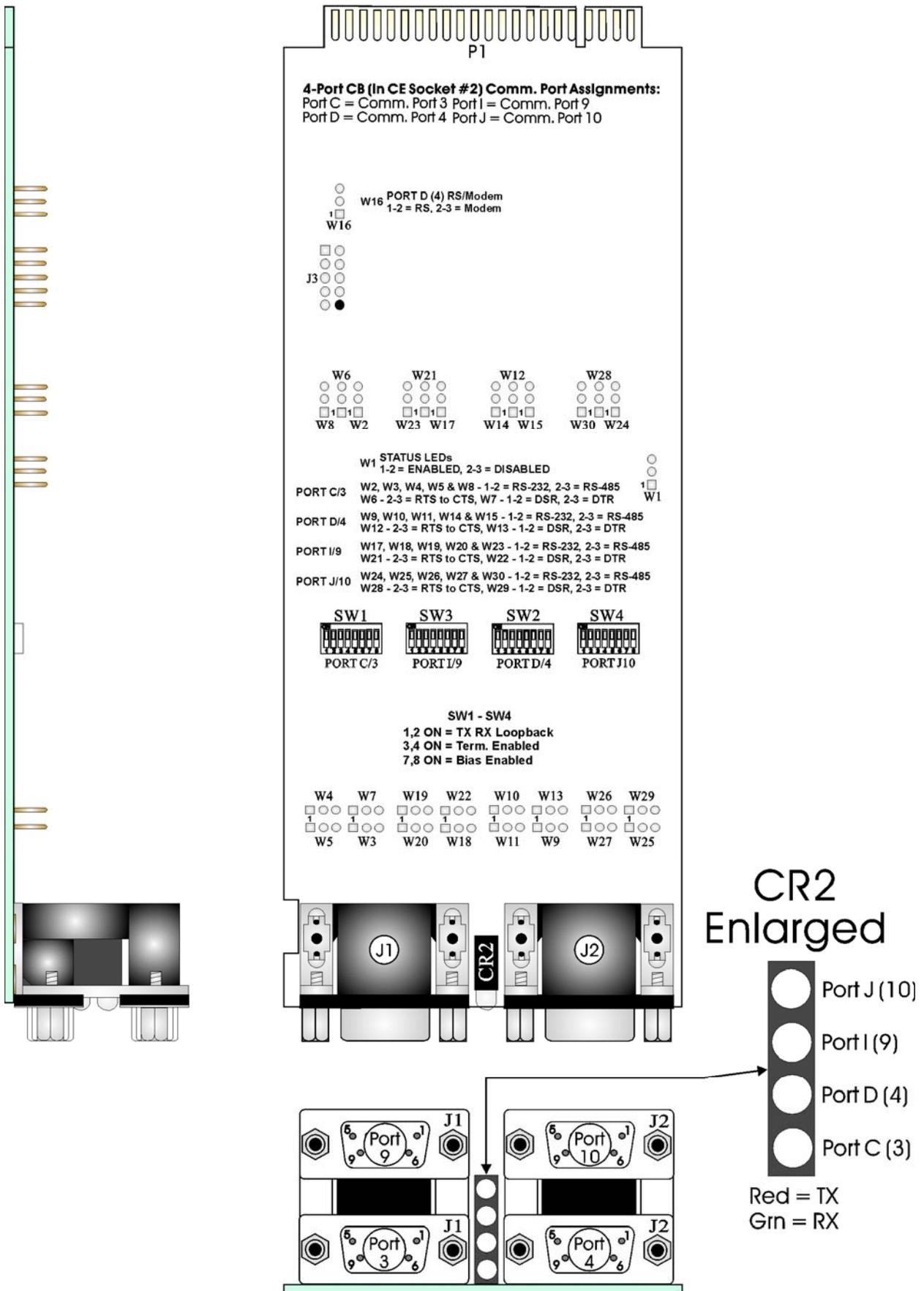
Figure 10 - CW\_35 - 4-Port CB Board Component Identification Diagram
