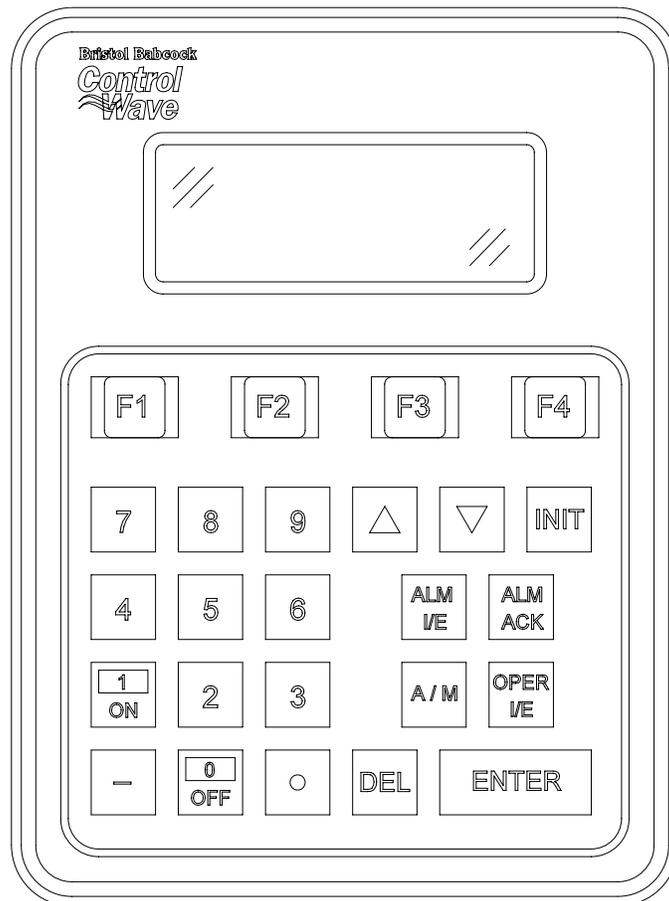
**Figure 1 - Display/Keypad Assembly – 25 Button Keypad & 4 X 20 Display**
