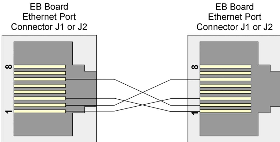
**Figure 6 - Point-to-Point 10/100Base-T Ethernet Cable**
