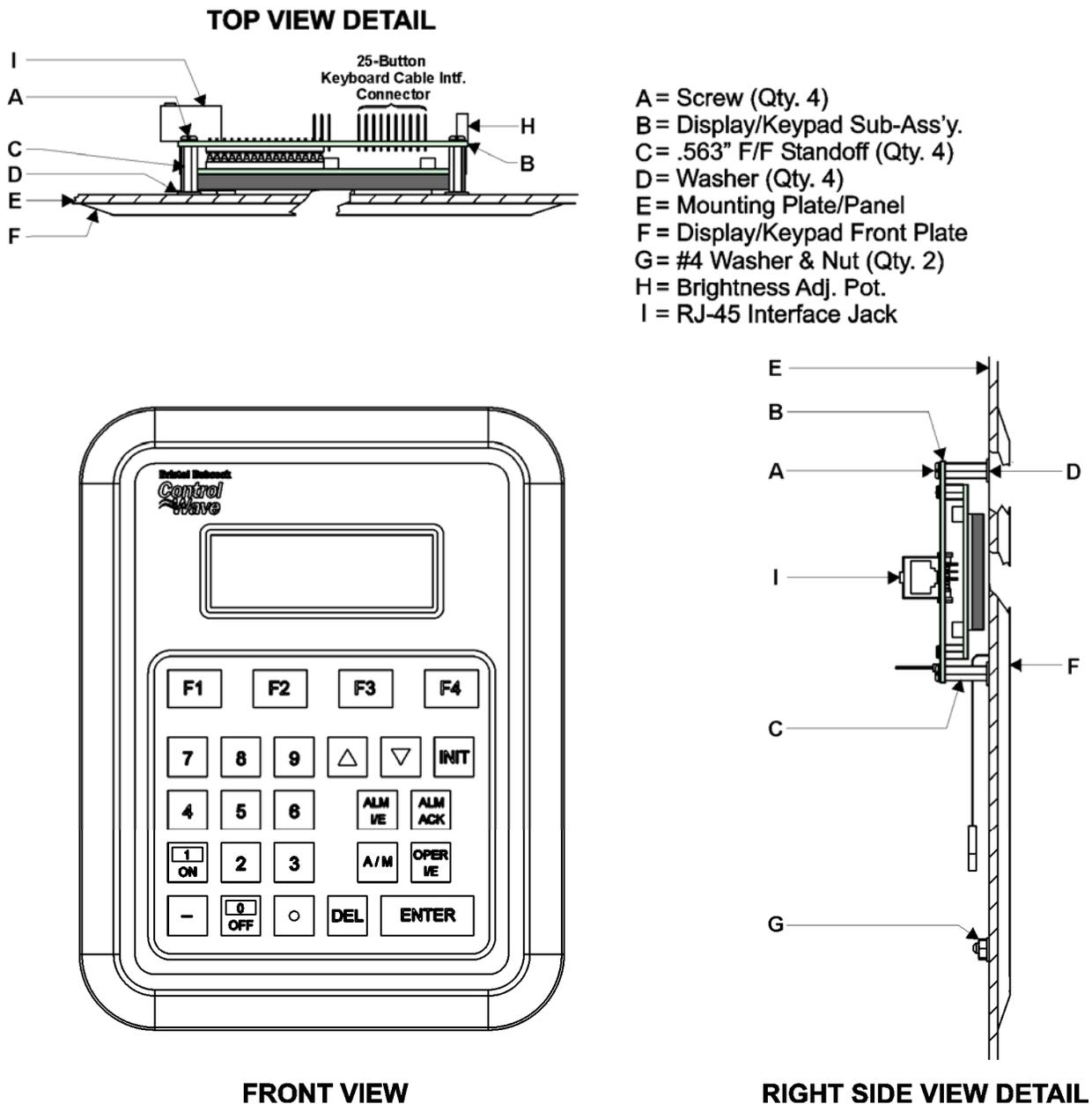
Figure 2-30 - 25-Button Display/Keypad Assembly Installation Drawing
