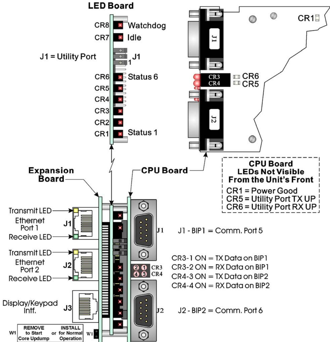
**Figure 4 – CW\_35/31 CPU Module LED Identification**
