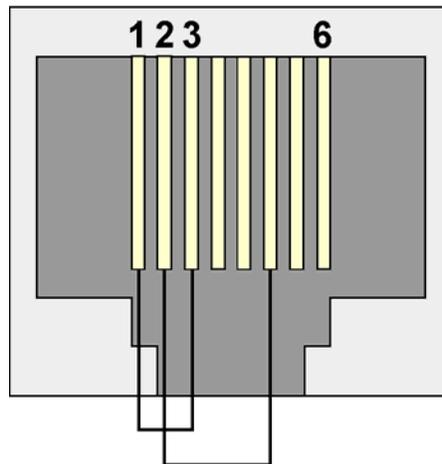
**Figure 8 – 10/100Base-T Connector (P2) with Cable Configured for Loopback**
