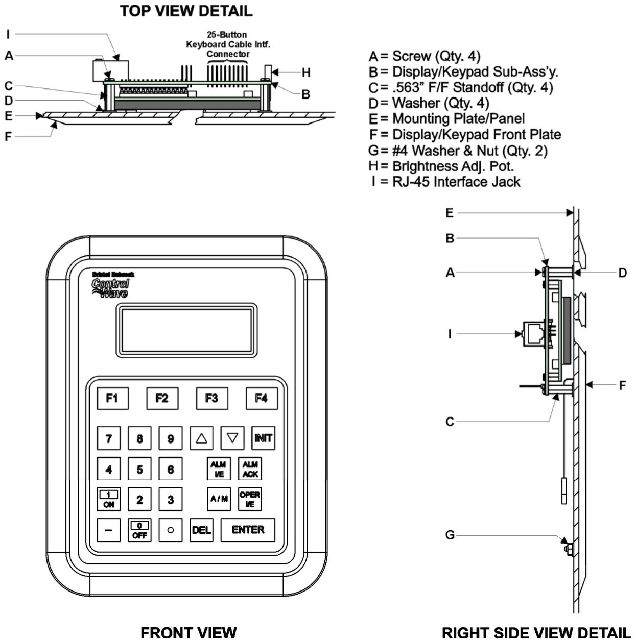
Figure 14 - 25-Button Display/Keypad Assembly Installation Drawing
