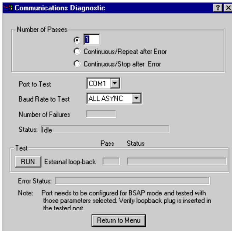
**Figure 26 - WINDIAG’s Communications Diagnostic Menu**
