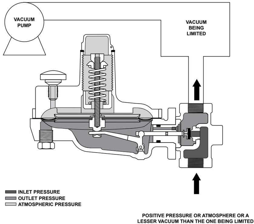
Figure 2. Type Y690VB Operational Schematic
