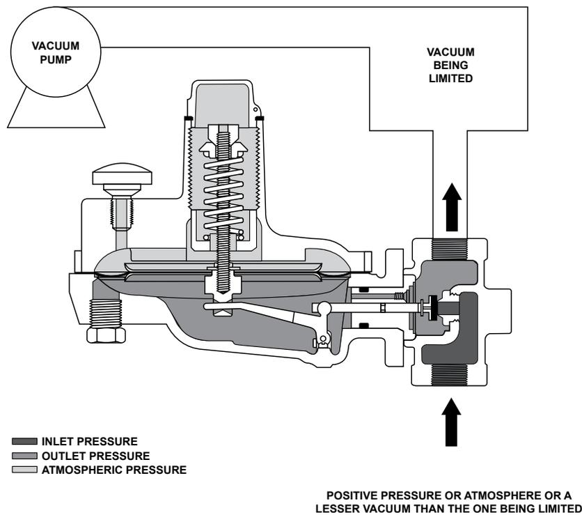
Figure 2. Type Y690VB Operational Schematic
