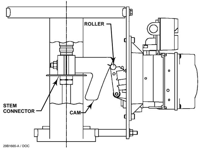
Figure 4-7. Feedback Connection for Typical Long-Stroke Sliding-Stem Actuator (4 to 24 Inches Travel)
