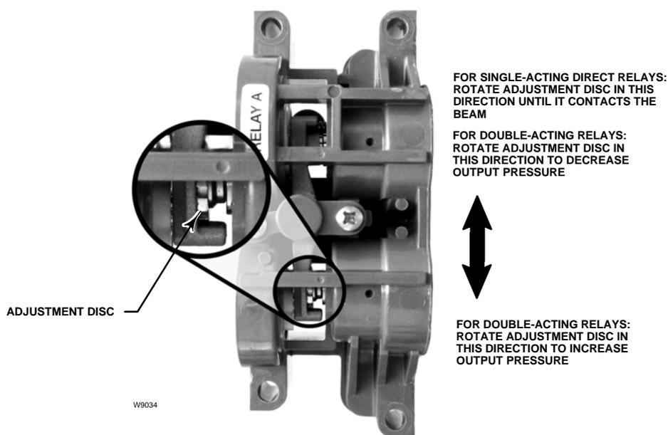
Figure 5-2. Relay A Adjustment (Shroud Removed for Clarity)
