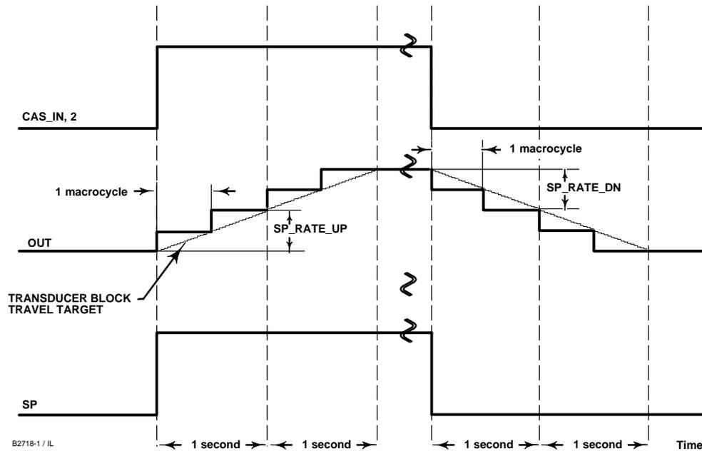
Figure 4-10. Analog Output Function Block Timing Diagram
