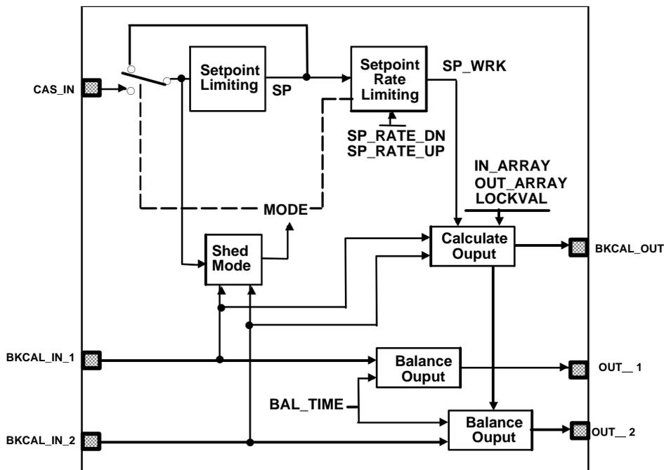
Figure 4-19. Output Splitter Function Block Schematic Diagram
