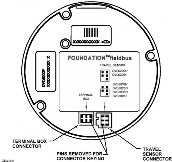
Figure 7-2. Back View of PWB Assembly Sub-Module
