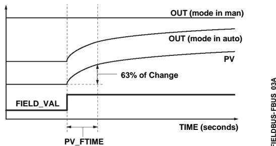
Figure 4-25. Analog Input Function Block Timing Diagram
