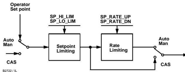
Figure 4-13. PID Function Block Set Point Selection
