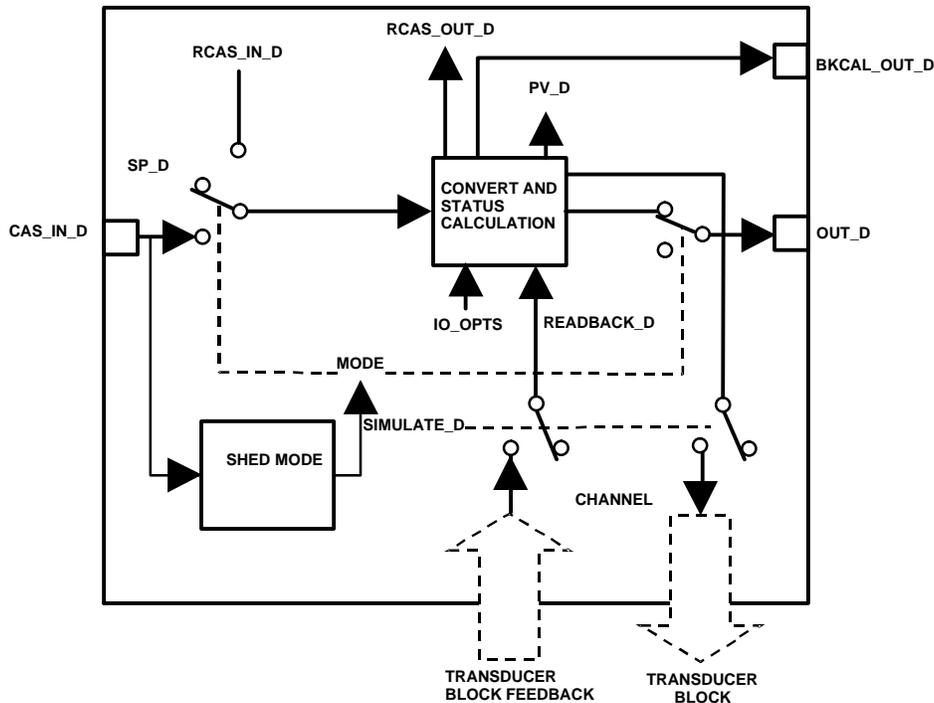
Figure 4-29. Discrete Output Function Block Schematic
