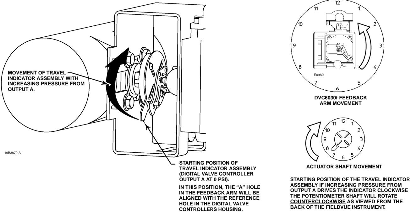
Figure 2-10. Explanation of FIELDVUE DVC6030f Travel Indicator Starting Position and Movement if **Counterclockwise** Orientation is Selected for "Travel Sensor Motion" in ValveLink Software or the Field Communicator
