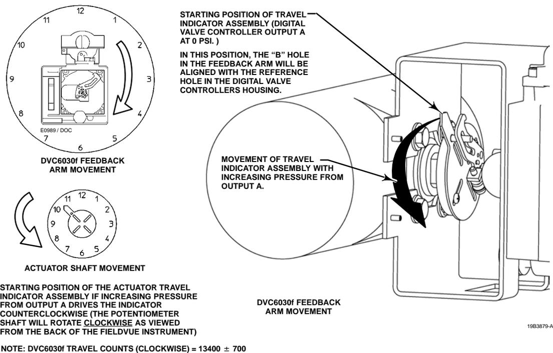
Figure 2-9. Explanation of FIELDVUE DVC6030f Travel Indicator Starting Position and Movement, if **Clockwise** Orientation is Selected for "Travel Sensor Motion" in ValveLink Software or the Field Communicator
