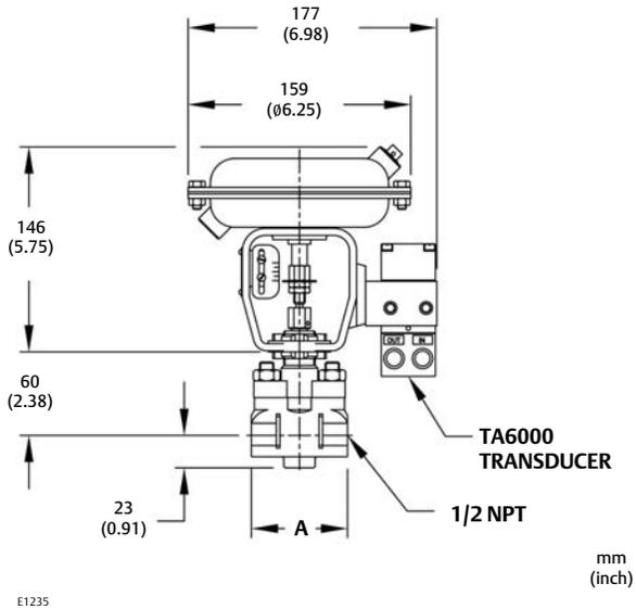
Figure 8. Baumann 16 Actuator with TA6000 (Top View)
