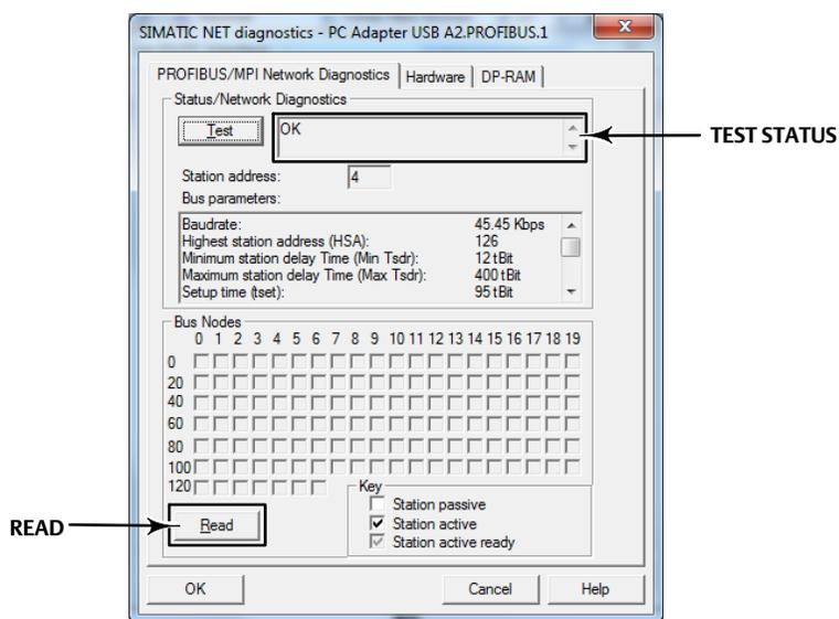
7. Any master or slave (devices) that is connected will be reflected (in the example shown in figure 7, the PROFIBUS card is connected to address 4). Station Active refers to Masters on the bus. Station Passive refers to the slave (devices) on the bus. An active ready PLC (Master Class 1) will be denoted as Station Active Ready.
