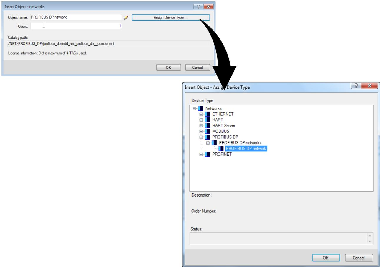
5. A new network now appears on the right pane, as shown in figure 14. Right-click on the network and select Insert New Object > Object.
