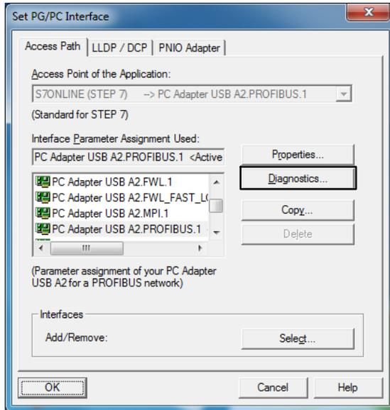
4. In the Diagnostics window, shown in figure 5, click on Test to check the status of the PROFIBUS card and network.
