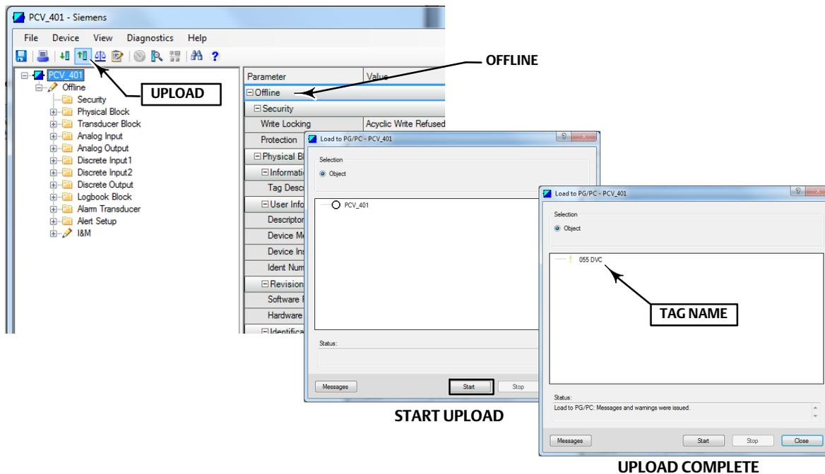
The project is now setup, and you are able to communicate with the DVC6200p. Proceed to Going Online with the DVC6200p on the next page.
