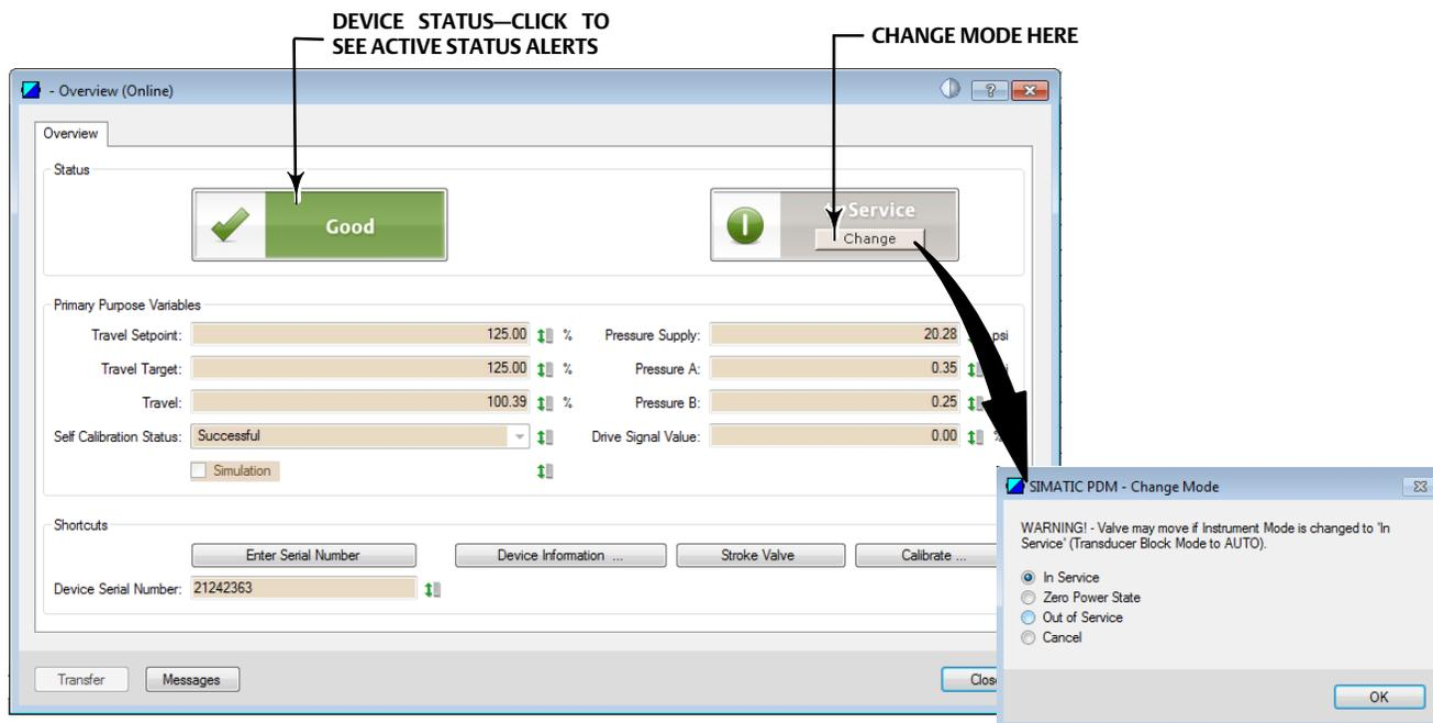
2. To configure the DVC6200p, select Configure > Guided Setup and go to Device Setup as shown in figure 20. Follow the prompts to configure actuator and valve information, calibrate, and tune the valve assembly. If Device Setup is being done prior to mounting the device, refer to the note on the following page.
