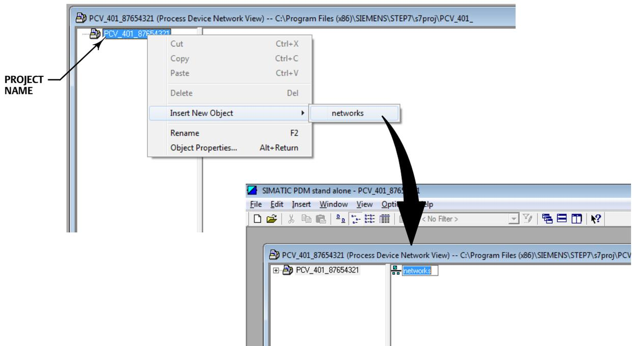
3. Right click on the networks icon in the right pane and select Insert New Object > Communications Network as shown in figure 12.
