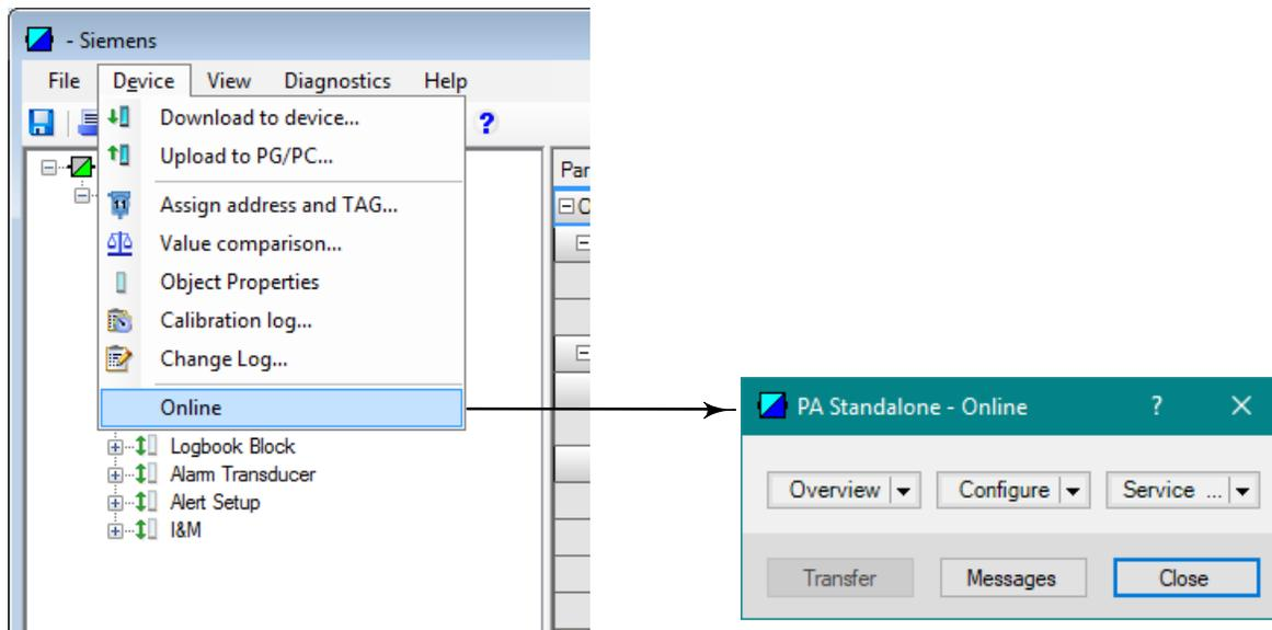
Refer to figure 19 to view the Overview screen interface. Overview shows the Primary Purpose Variables and the Device Status and Mode. It also allows you to enter the Device Serial Number and access Device Information, Stroke Valve, and Calibration procedures.
