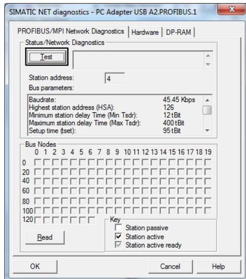
5. Confirm the status is OK (see figure 6.) If the status is Failed, changes to the parameters set in step 2 may be required.
