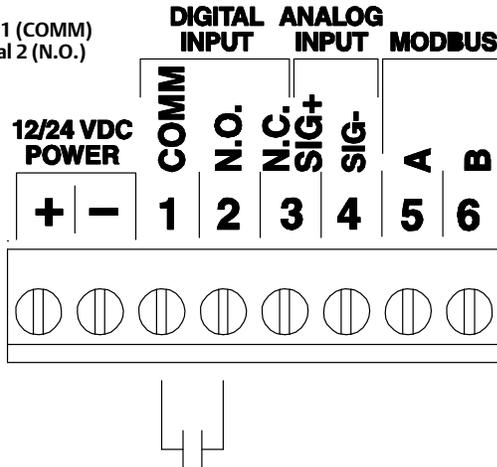
Figure 7. Wiring - Modbus Input
