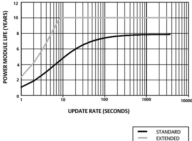
NOTE: THREE SUB-DEVICES ARE ASSUMED, CONSTANT TEMPERATURE OF 22°C (72°F).
