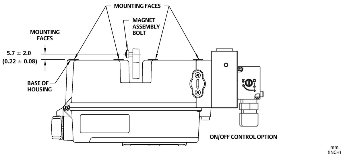
Figure 11. Housing and Mounting for Linear and Quarter-Turn Actuators
