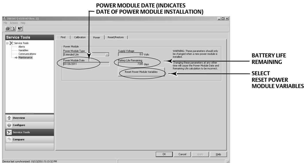
1. A warning will be displayed, noting this should only be done when a new power module is installed. Select Next if you have replaced the power module. Select Cancel if the power module has not been replaced.
