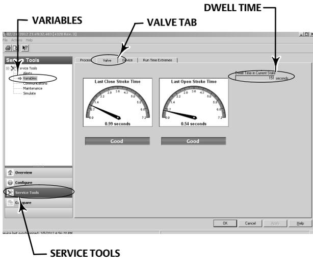
Figure 29. Viewing Dwell and Transition Dwell Times in AMS Wireless Configurator and AMS Device Manager
