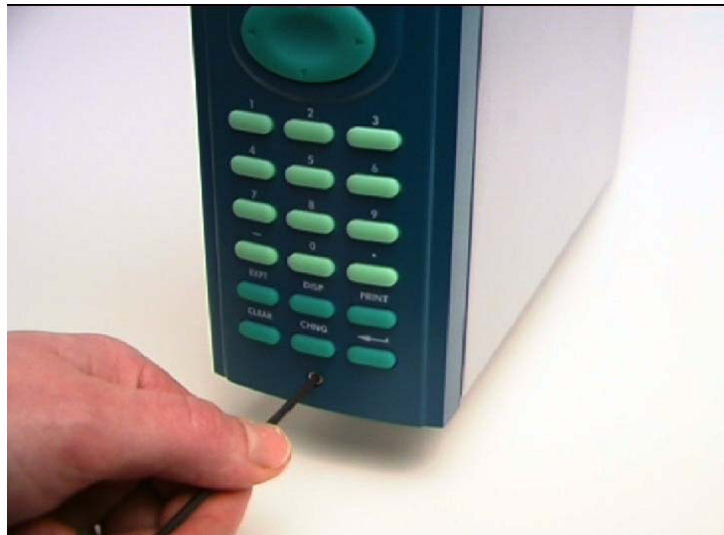
Figure 2-2. Removing the Front Panel
