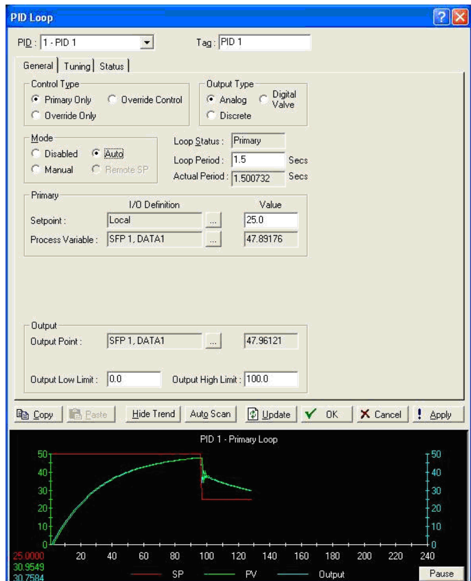
Figure 7-85. PID Loop - Show Trend/Hide Trend
