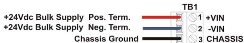
Figure 2-11. Wiring System Power to the PSSM
