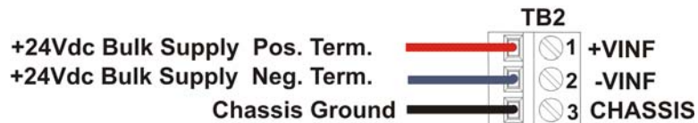
Figure 2-12. Wiring Field Power to the PSSM
