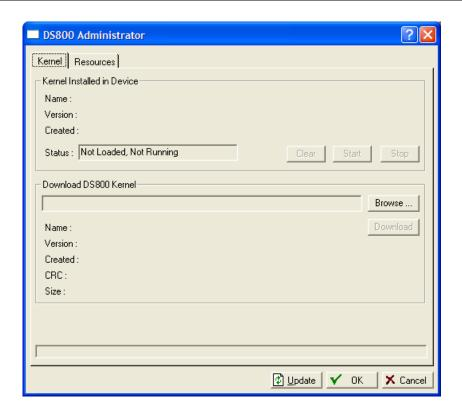
Note: This screen has two tabs: Kernel and Resources. Use the Kernel tab to load the DS800 kernel and view associated information. Use the Resource tab to load binary DS800 programs without the PC-based Workbench software. The upper frame on the Kernel tab (Kernel Installed in Device) provides information on the kernel currently installed; the lower frame identifies and provides specific information on kernels you may want to download to the FB107.
