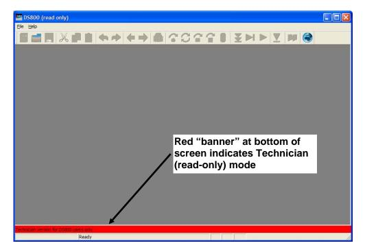
The red banner at the bottom of the DS800 screen indicates that the software successfully installed but was unable to find the license key.
