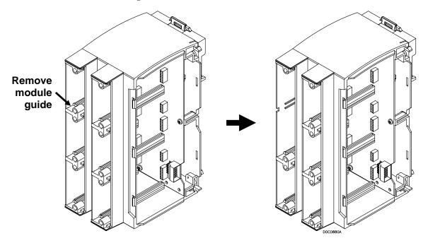
Figure 1. Original and Converted Series 2 Expansion Backplane
