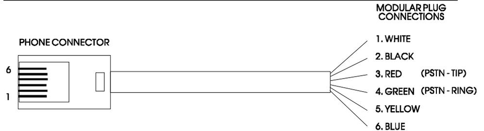
*Figure 3-8. Wiring for Phone Connector*
