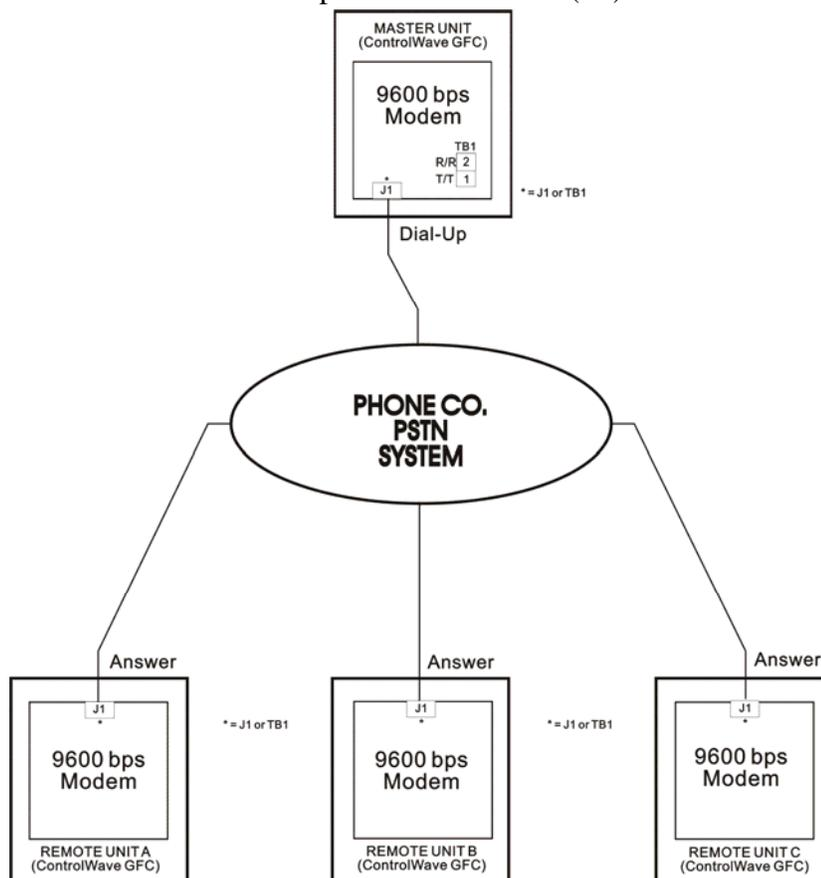
Figure 1-1. Typical 9600 BPS - PSTN Modem Network
