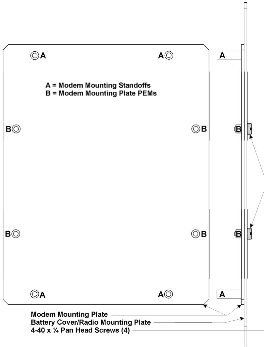
Figure 3-1. Modem Mounting Plate and Battery Cover/Radio Mounting Plate (GFC, Corrector, EPAC)
