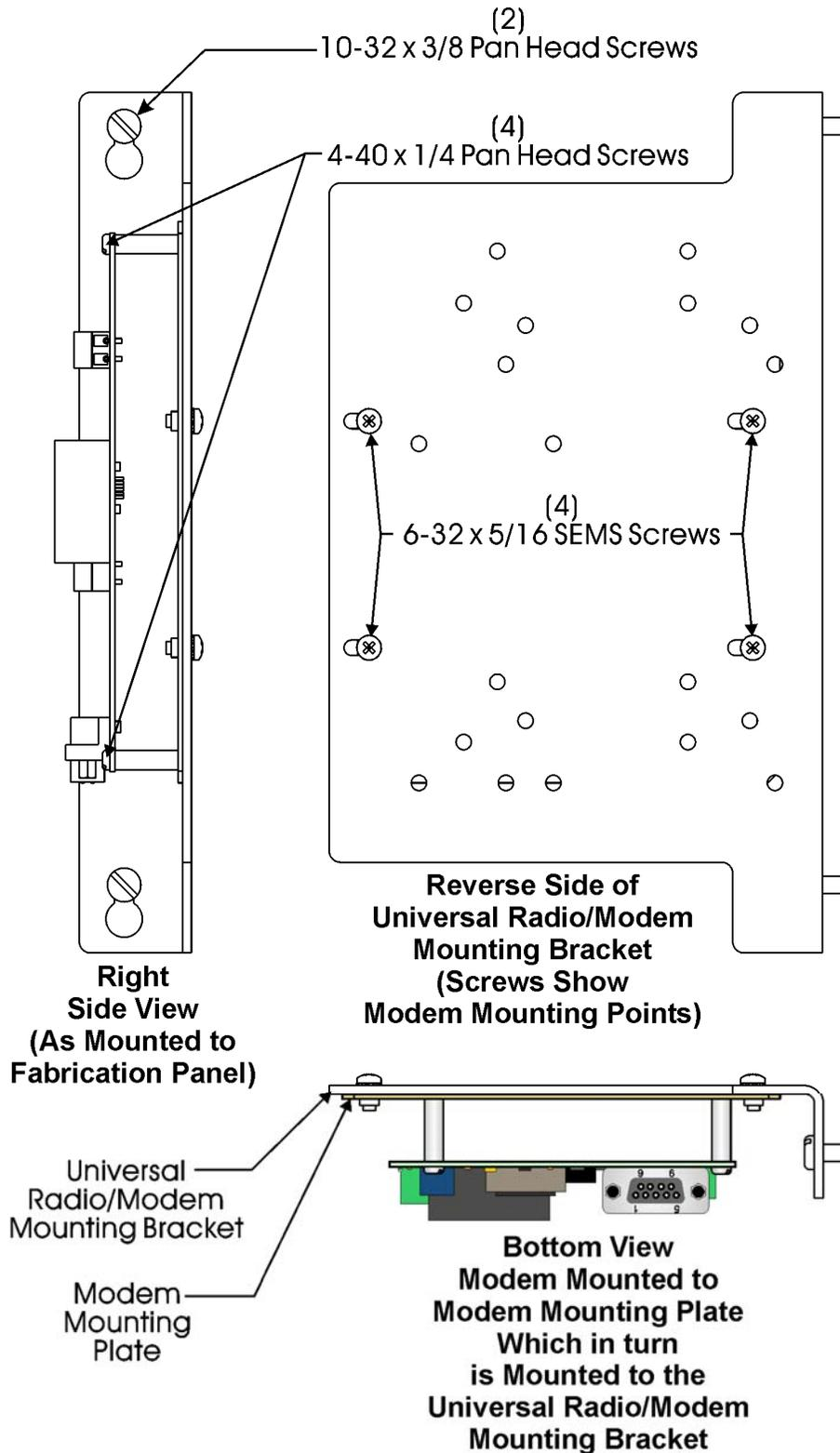
Figure 3-6. Modem Installation Diagram (GFC Plus) - Modem mounted to Modem Mounting Plate, Modem Mounting Plate mounted to Universal Radio/Modem Mounting Bracket which in turn is mounted to the Fabrication Panel
