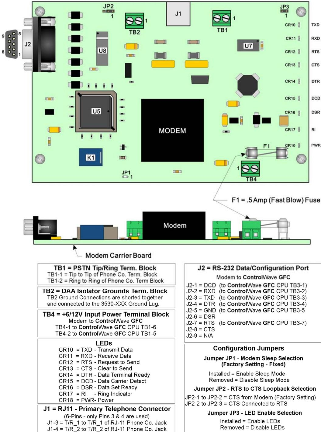
Figure 1-2. 9600 PSTN Modem Assembly - P/N 400000-01-6
