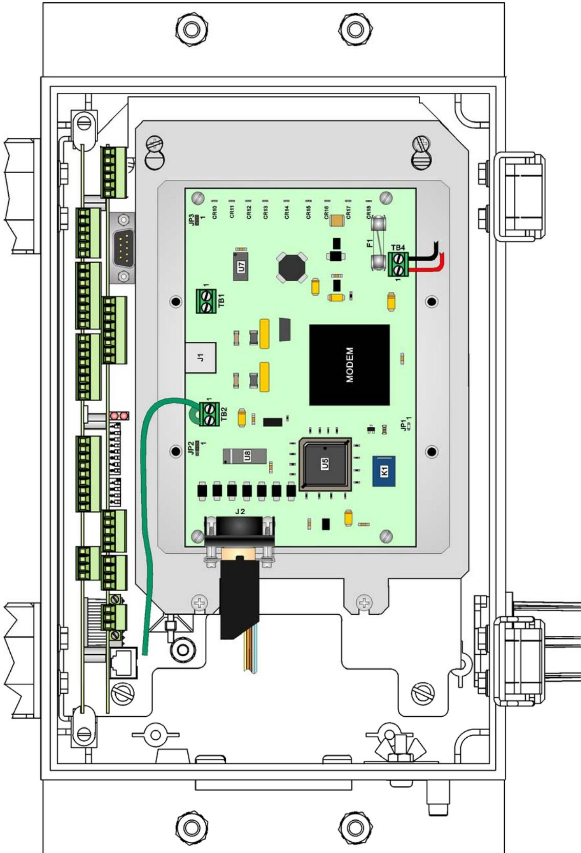
Figure 3-5. 9600 PSTN Modem Installed in ControlWave EPAC (Front View)
