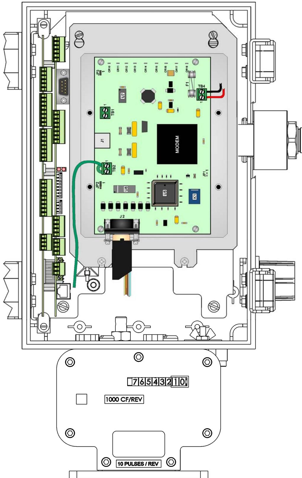
Figure 3-4. 9600 bps - PSTN Modem Installed in ControlWave Corrector (Front View)
