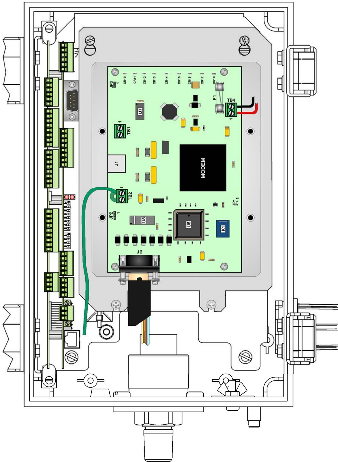
Figure 3-3. 9600 bps - PSTN Modem Installed in ControlWave GFC (Front View)
