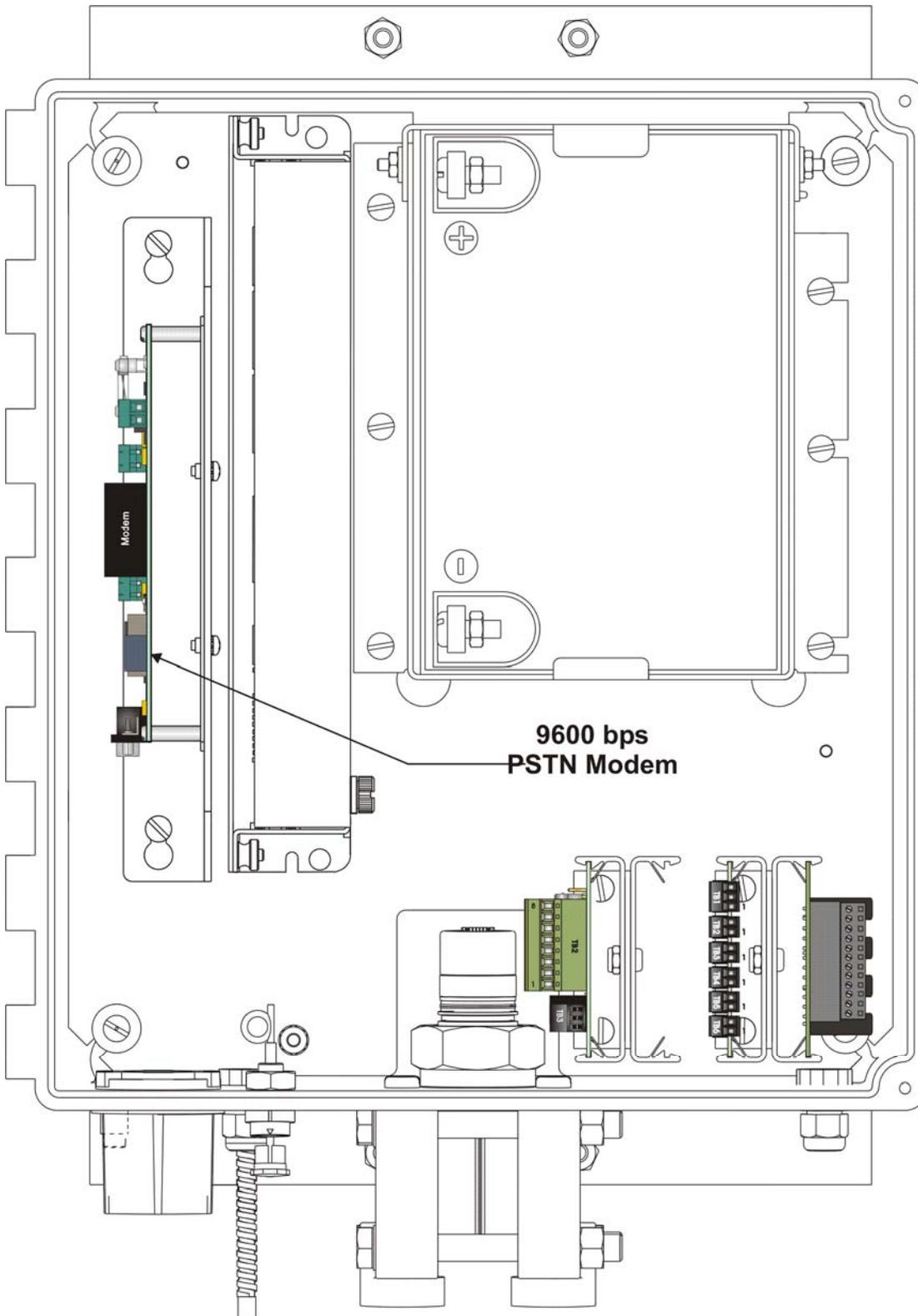
*Figure 3-7. 9600 bps - PSTN Modem Installed in ControlWave GFC Plus (Front View)*
