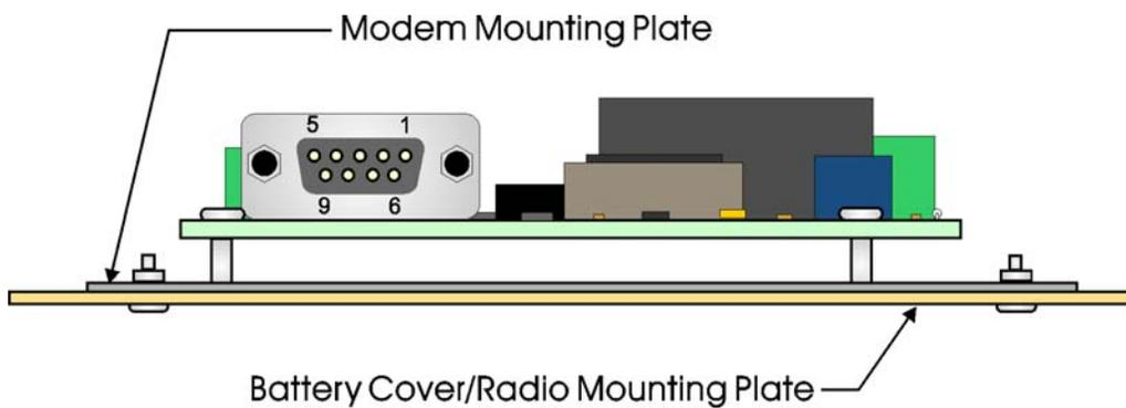
Figure 3-2. Modem Installed on Battery Cover/Radio Mounting Plate (GFC, Corrector, EPAC)
