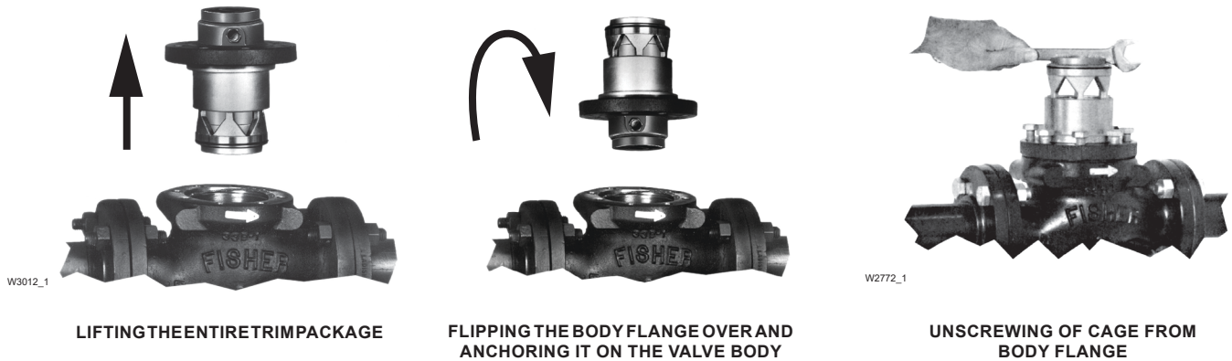
Figure 10. Replacing Trim Parts on Site Using Body as Holding Fixture
