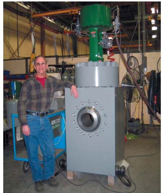
This is one of two identical, block-body Fisher® valves featuring five-stage Cavitrol® IV trim. The 16,000-pound assembly was hydro-tested at 13,000 psig. Its trim was designed to stage the pressure drop, separate shutoff and throttling, and prevent erosion.
