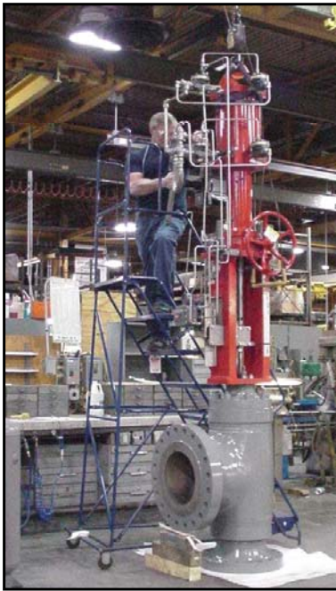
Figure 2: 16" Compressor Antisurge Valve
