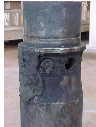
Figure 2: DST Trim After Four Years of Service
