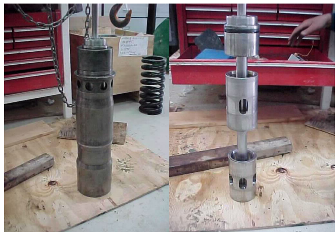
Figure 3: DST Trim Prior to Reinstallation
