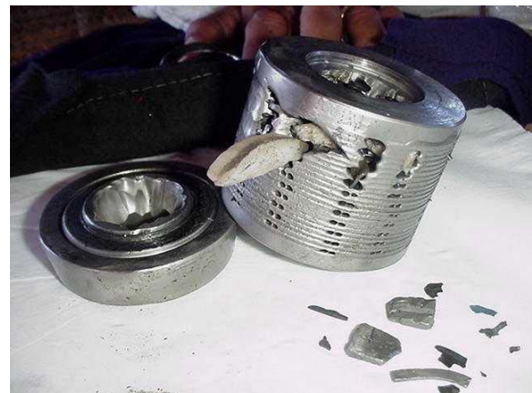
Figure 1: Damaged Tortuous Path Trim
