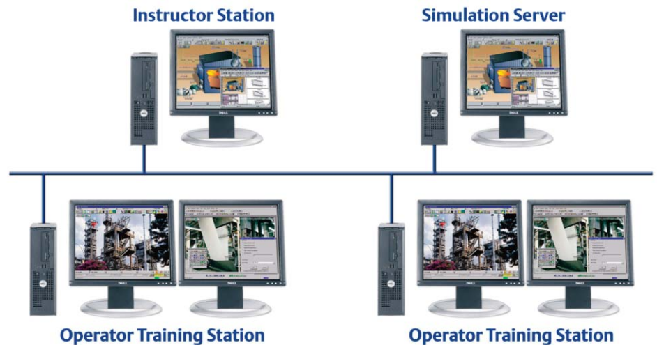
DeltaV™ Simulate Training Solution Architecture
