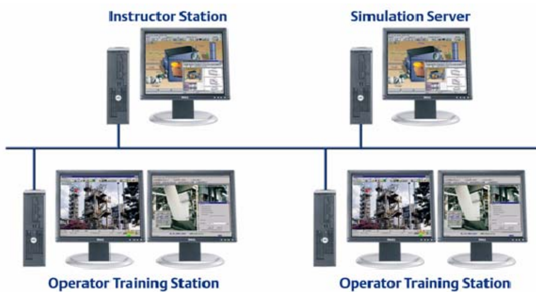
Multiple DeltaV Simulate “Standalone” workstations networked to a simulation server. The number of operator training stations can vary from 1 to 32.
