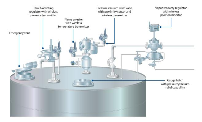
Emerson provides the widest array of environmental protection and safety equipment, expertise and unparalleled service across a full range of oil and gas, chemical and other industries worldwide. Rely on our expertise to help you create a total tank solution that may include tank blanketing, vapor recovery, pressure vacuum relief, flame protection and more.
