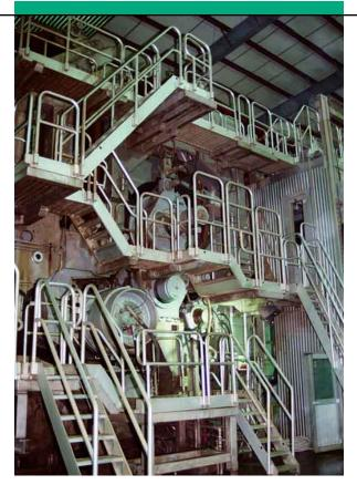
Pratt installed an OVER Meccanica four-drinier type board machine at the Shreveport mill to produce high performance, lightweight linerboard from 100% recycled paper.
