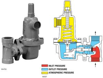
Figure 1. Type 627 Direct-Operated Regulator and Operational Schematic
