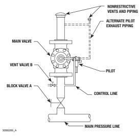
**RELIEF PRESSURE CONTROL AT RELIEF VALVE INLET**
