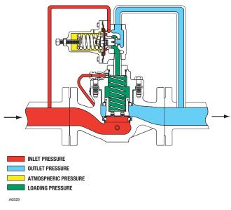
Figure 3. Type 63EG Backpressure Regulator/Relief Valve Operational Schematic
