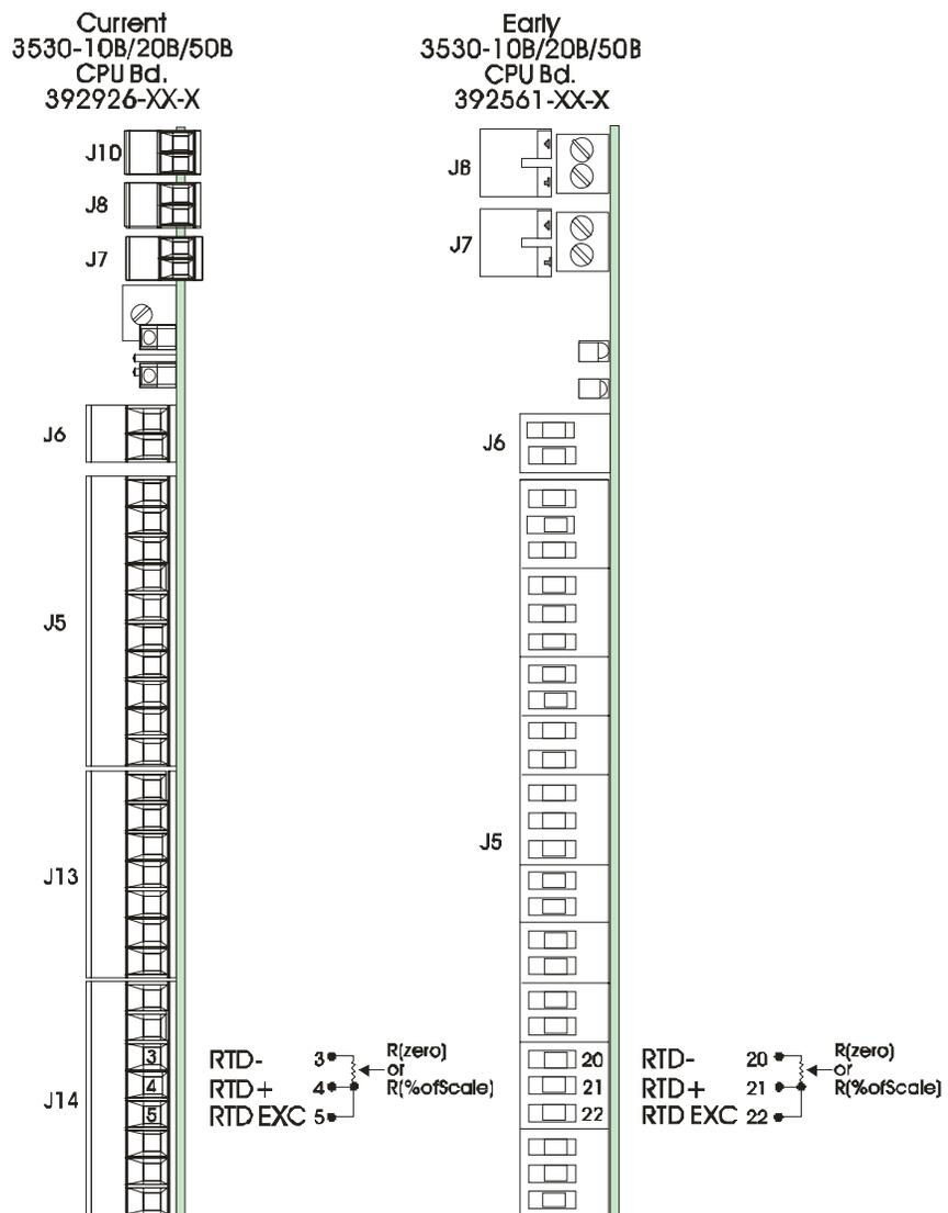
Figure 8-4. TeleFlow CPU Board RTD Calibration Connection Diagram (See page 5-7 for resistor values)
