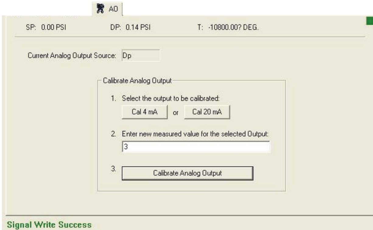
Figure 7-7. AO tab – Calibrating the Analog Output
