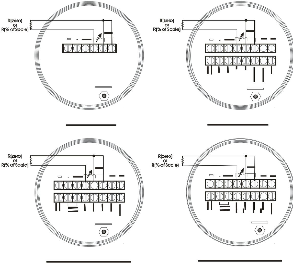
Figure 6-4. Model 3508 TeleTrans - Connections for RTD Calibration (See page 5-7 for resistor values)
