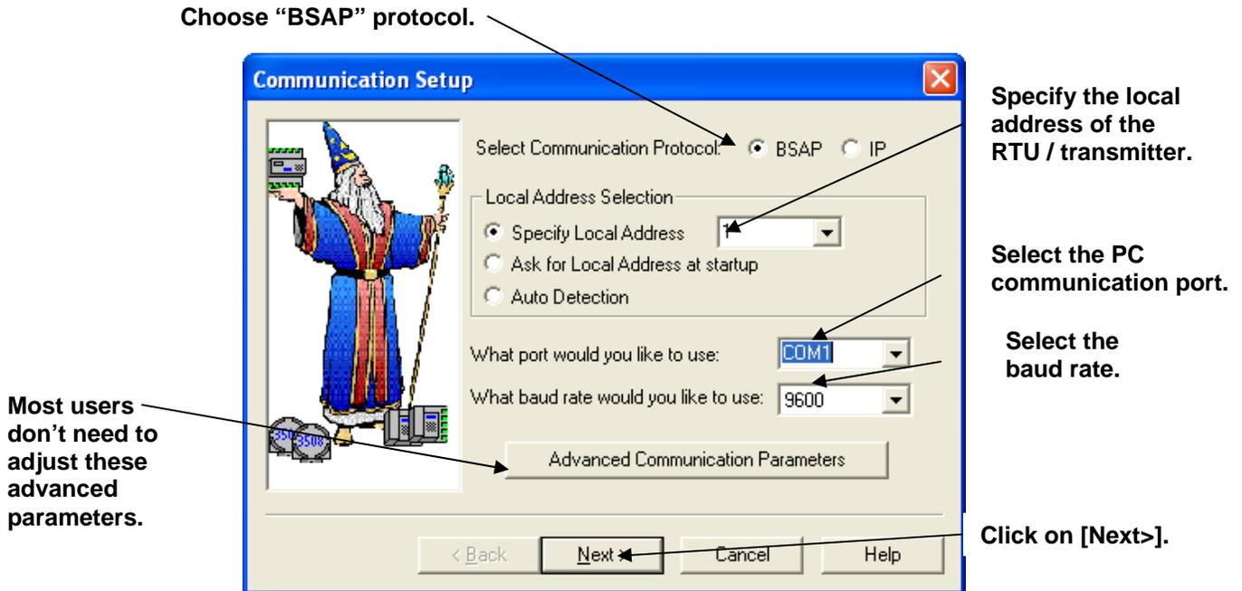
Figure 3-2. Communication Setup dialog box (BSAP)
