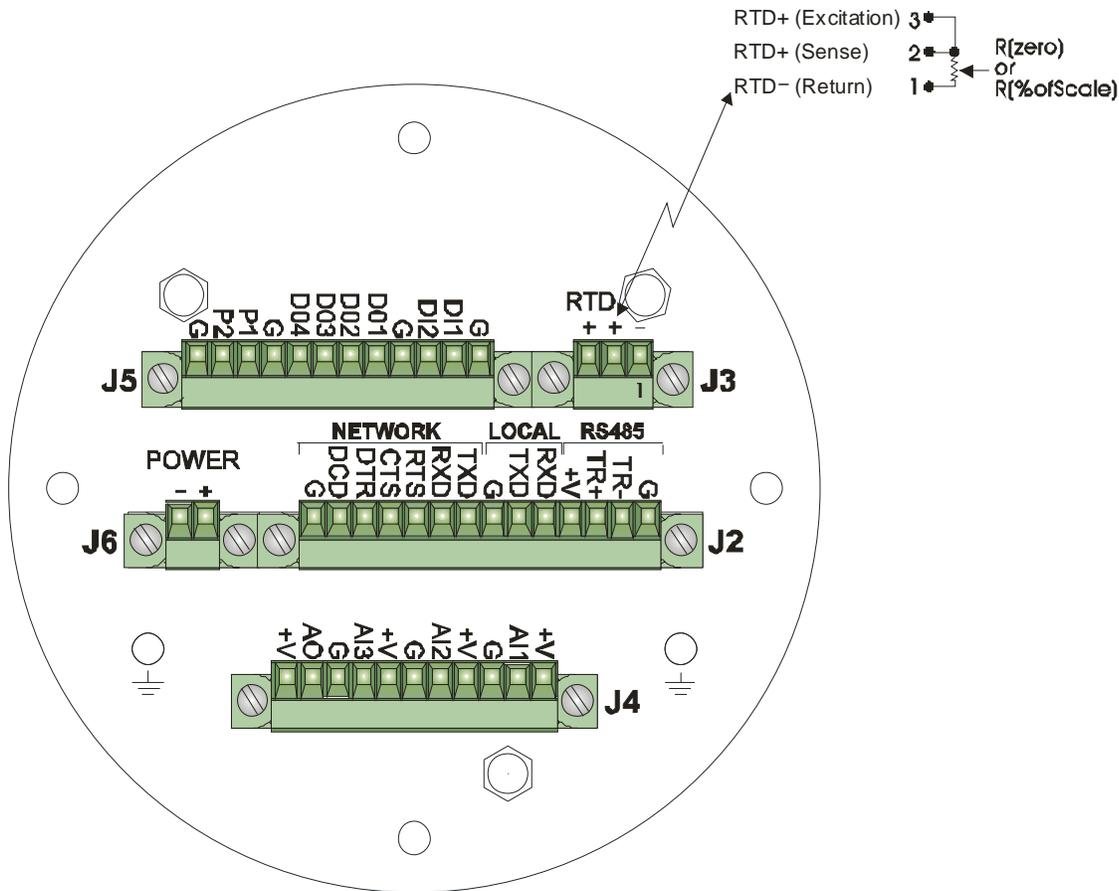
Figure 9-7. Connections for RTD Temperature Calibration – ControlWave XFC (see page 5-7 for resistor values)
