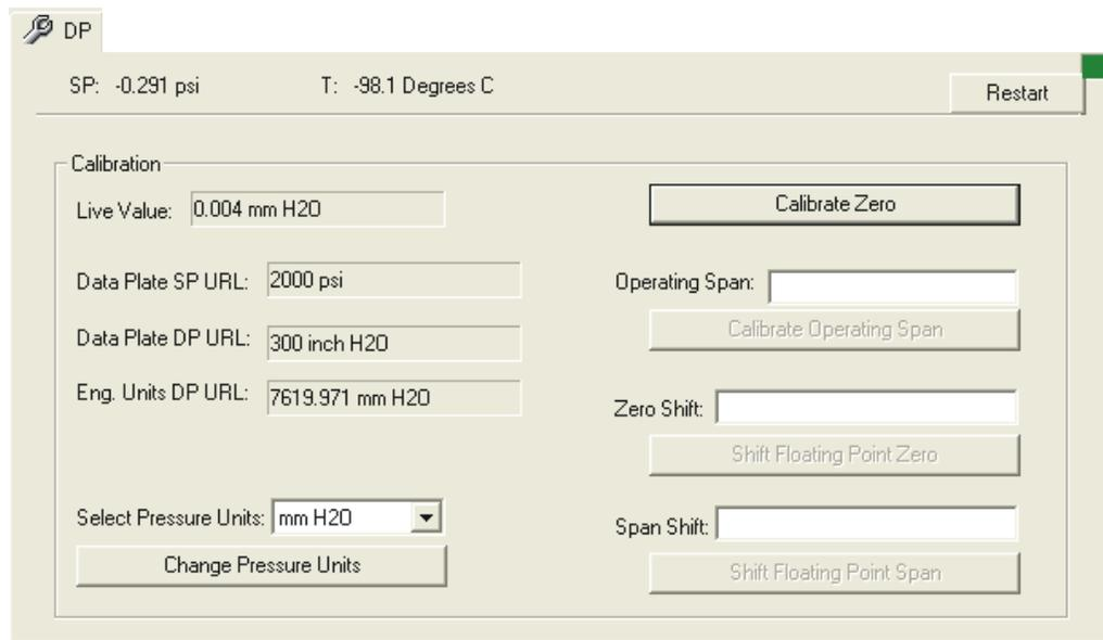
Figure 6-1. DP Tab – Calibrating Differential/Gage Pressure
