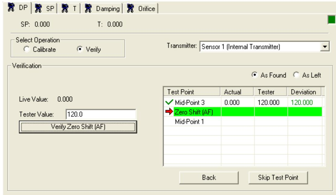
Figure 9-2. DP tab – Verification of Differential / Gage Pressure
