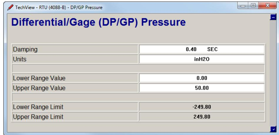
Figure 10-2. Configuring the Differential/Gage (DP/GP) Pressure Variable
