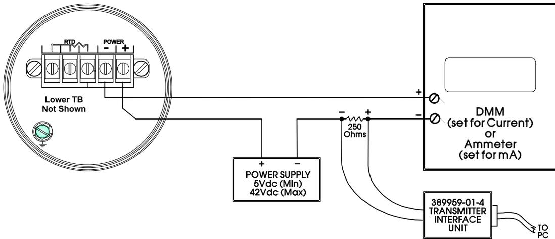
Figure 7-6. 3808 Analog Output Calibration - Current Measurement Diagram
