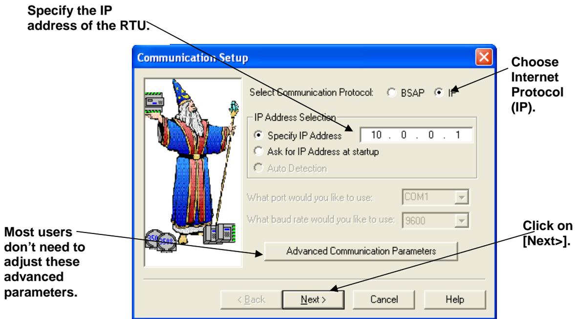
Figure 3-3. Communication Setup dialog box (IP)
