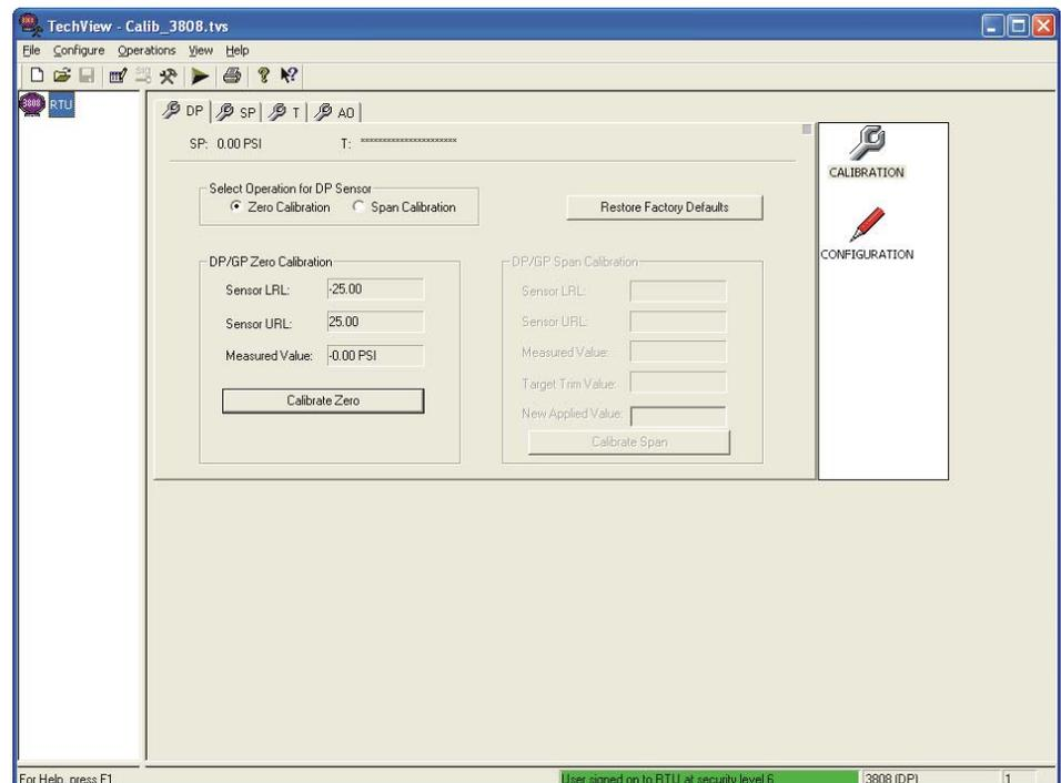
Figure 7-1. DP tab – Calibrating Gage or Differential Pressure
