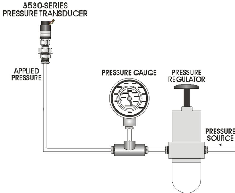
Figure 8-6. 3530-45B/-55B TeleRecorder Pressure Transducer Connections
