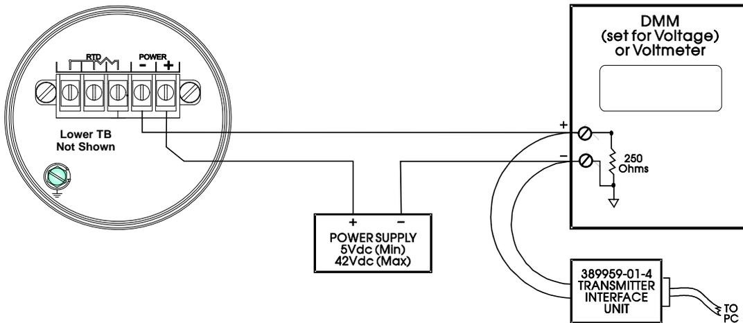
Figure 7-5. 3808 Analog Output Calibration - Voltage Measurement Diagram
