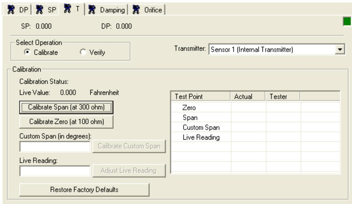
Figure 9-5. T tab - Calibration of RTD Temperature
