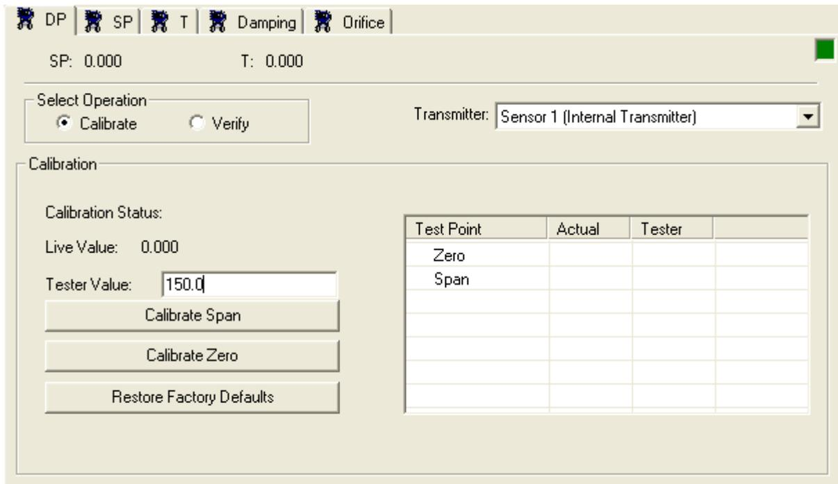
Figure 9-1. DP tab – Calibration of Differential / Gage Pressure
