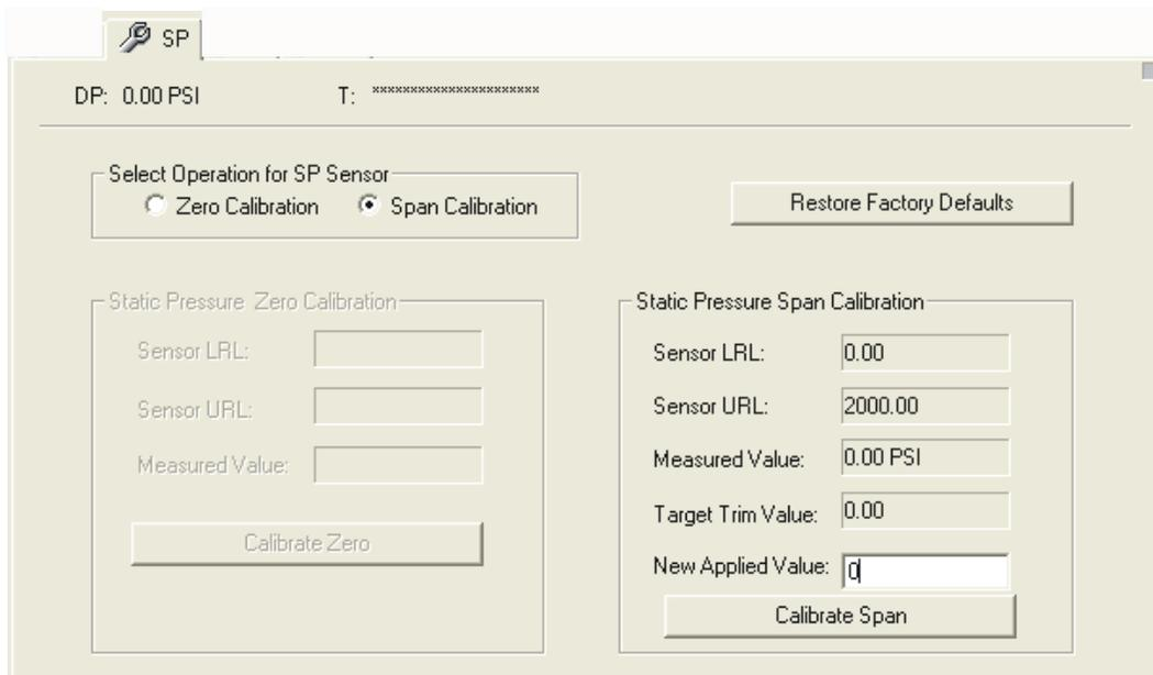
Figure 7-2. SP tab - Calibration of Station Pressure
