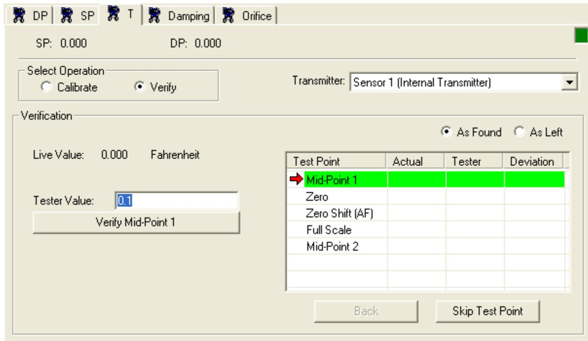
Figure 9-8. T tab – Verification of Temperature
