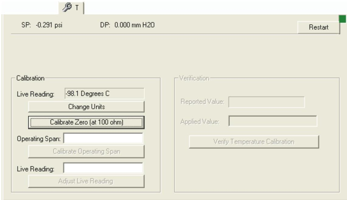
Figure 6-3. T tab – Calibrating RTD Temperature
