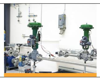
Team Fisher engineered a two-valve solution (like the one used in a differentiation lab (above) to meet severe-service requirements in a silane unit. Two eight-inch, Design ED valves with Inconel body-trim, full bellows, and FIELDVUE DVC6000-PD tier instruments serve a plant producing silicon
