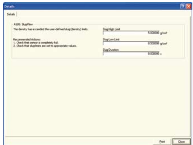
Advanced Coriolis flowmeters have diagnostics that can detect slug flow and guide operators and maintenance technicians towards corrective action.
