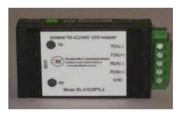
Instruction for using the datalink communications USB to RS485 converter with the ER3000
