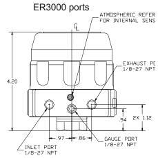
The ER3000 can be installed either directly on top of the regulator's air loader using the supplied adapter or using tubing between ER3000 outlet and regulator dome/air loader.
