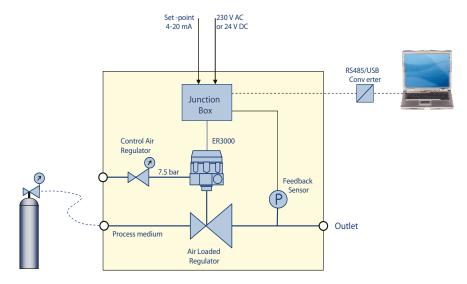
The set point can be either an analog 4 - 20 mA or 1 - 5 volt signal or an RS485 serial signal from a computer. A converter to change the signal to RS485 from RS232 or USB is available with the kit. The PID parameters can be fine tuned using the supplied Tescom software loaded on the PC. In the case of an analog set point, the PC connection is needed only once for optimizing the PID parameters.
