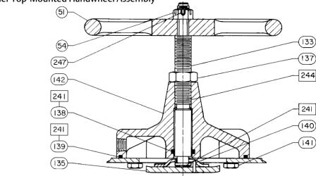
□ APPLY LITHIUM GREASE TO 241, ANTI-SEIZE LUBRICANT TO 244.
