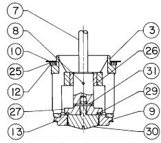
**EQUAL PERCENTAGE VALVE PLUG** 38.1 mm AND 50.8 mm (1.5 INCH AND 2 INCH) PORT DIÀMETER
