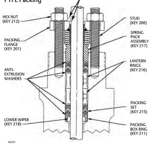
Figure 9. Typical ENVIRO-SEAL Packing System with **Duplex Packing**
