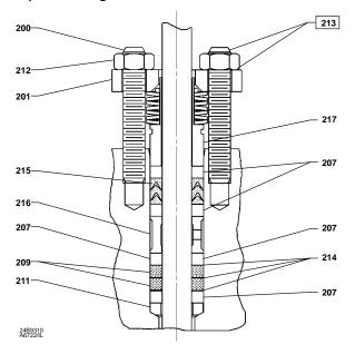
To For PTFE packing, tighten the packing box hex nuts until the top of the flange is even with the top of the sleeve on the follower (spring pack assembly).
