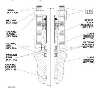
Figure 7. Typical ENVIRO-SEAL Packing System with PTFE Packing
