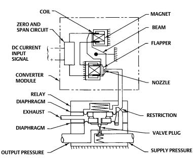
Figure 8. Fisher 646 Transducer Schematic
