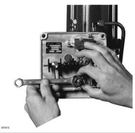
Figure 18. Proper Cam Position
