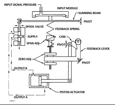
The 3710 pneumatic positioner accepts a pneumatic input signal and the 3720 electro-pneumatic positioner accepts a milliampere (mA), direct current (DC), input signal from a control device. The 3720 positioner uses a 3722 converter to provide a pneumatic input to the pneumatic portion (3710) of the electro-pneumatic positioner.
