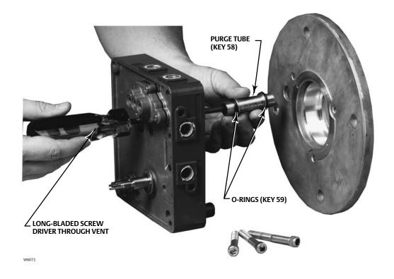
The positioner does not have an external vent connection. A unit exhausts actuator pressure through a screened hole (vent opening, figure 12) located in the positioner base plate. Do not restrict the vent opening. Restricting the vent opening can produce a pressure buildup in the positioner case and degrade positioner performance.
