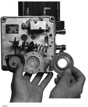
Figure 29. Assembly of Input Module
