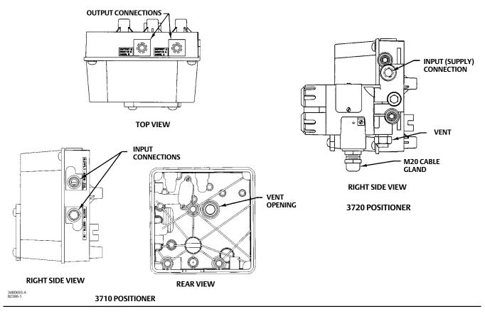
The conduit connection to the converter is 1/2-14 NPT.
