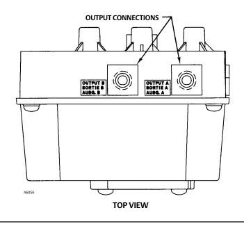
Use 3/8-inch tubing between the positioner and actuator.
