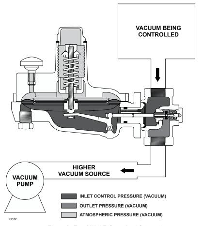
Figure 2. Type Y695VR Operational Schematic
