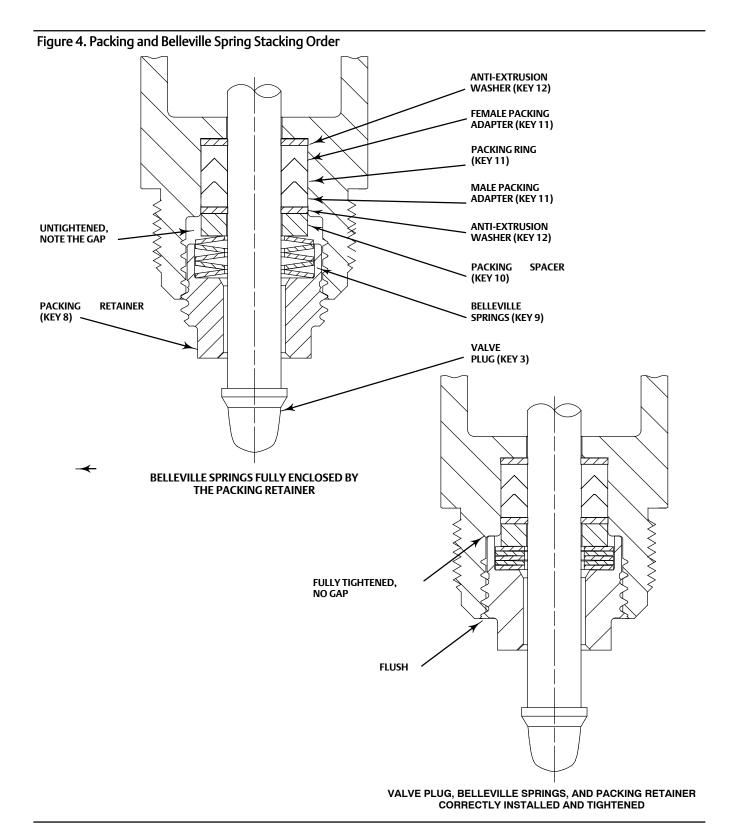
5. Install the male packing adaptor, lower anti-extrusion washer (key 12), and packing spacer over the valve stem as shown in figure 4.
